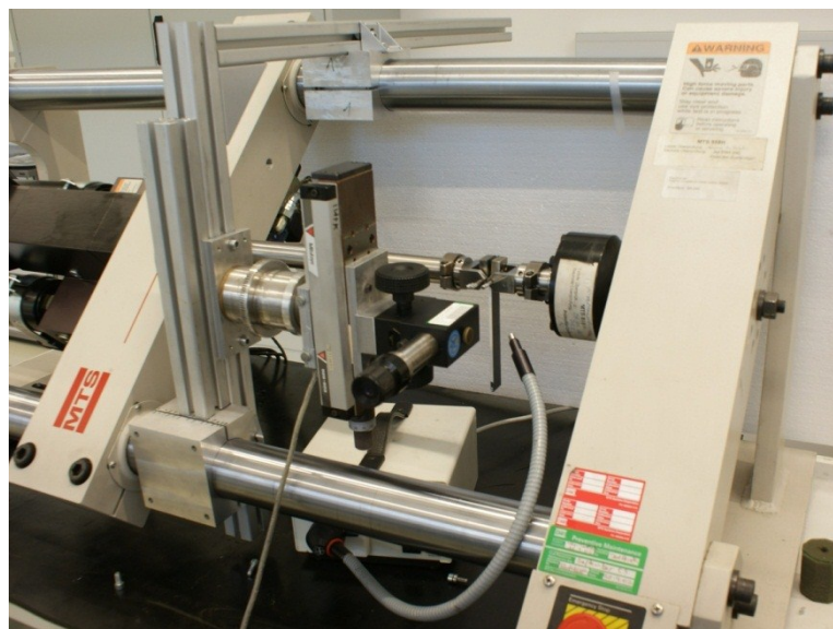
Figure 3.14: MTS 858, servo-hydraulic tabletop system with test setup for G_I -constant tests.
