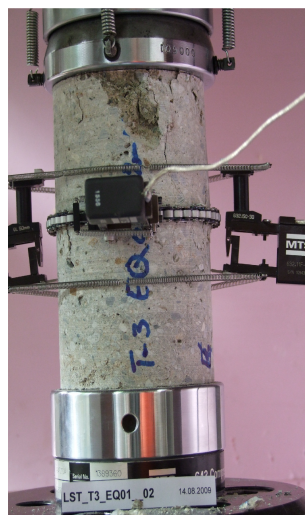
Figure 2.5: Uniaxial compression testing of the shotcrete sample using MTS test equipment
