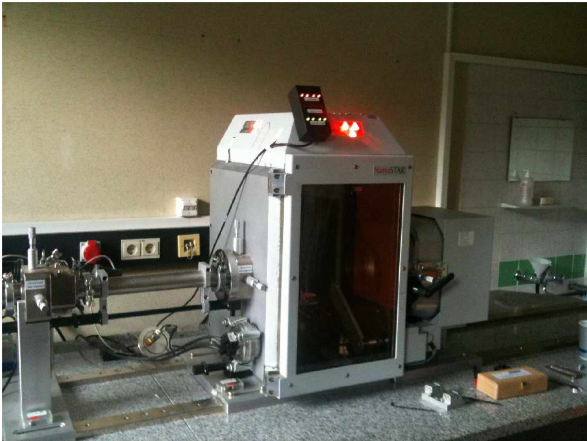
Fig. 3.4: Bruker NanoSTAR (Bruker AXS, Karlsruhe, Germany) small angle X-ray scattering (SAXS) equipment
