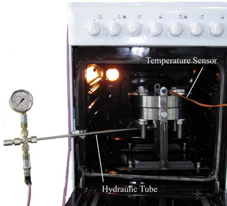
Figure 32: Measurement setup for increased temperatures
