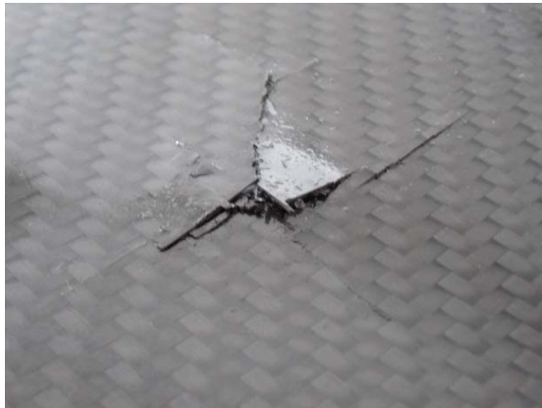
Figure 39: Burst 3mm coupon
