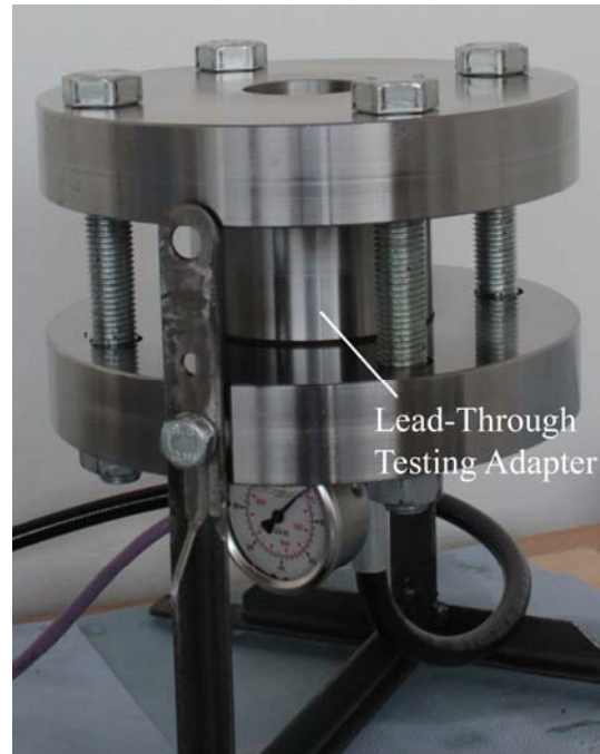
Figure 37: Fully assembled testing adapter for reverse pressure testing
