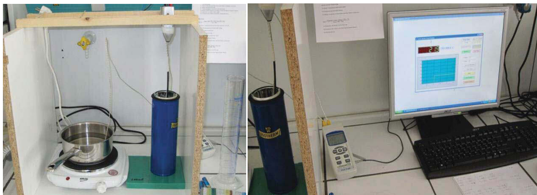
Figure 3-4: Liquid calorimeter for determining specific heat capacity
