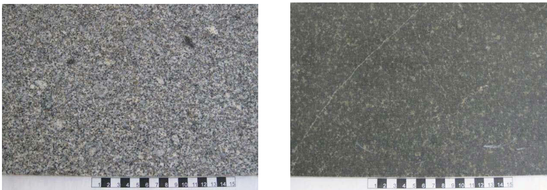
Figure 2-2: Two selected samples from the Lithothek: Granite (left) and Gabbro (right)
