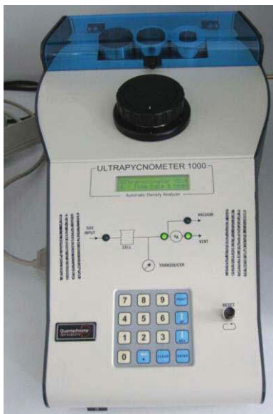
Figure 3-7: Helium pycnometer for grain density determination
