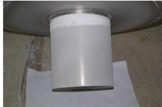
(b) Vortex finder outside with the three regions of depositions: a clean ring, thick depositions, thin depositions ( V600_{\mu_e 3.0} ).
