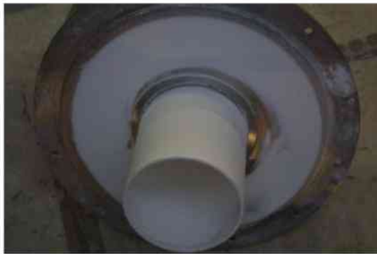
(c) The cyclone's roof covered with a closed ring of depositions ( V600_{\mu_e 2.0} ).
