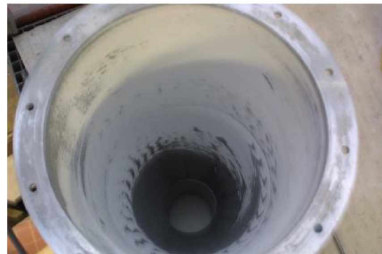
(f) Almost full covered cyclone body with "chevron shaped" depositions ( V600_{\mu_e 2.0} ).
