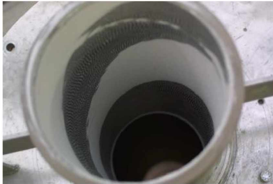
(a) Vortex finder inside with a helix of thick depositions on an underlay with a pattern of thin lines ( V600_{\mu_e 1.0} ).
