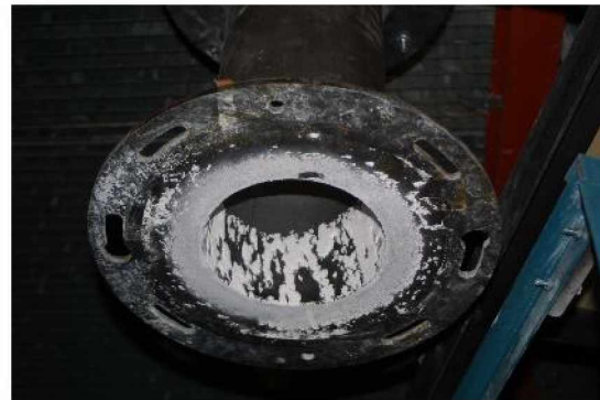
(d) Vertical tube section and flange with thick, stained depositions ( V600_{\mu_e 3.0} ).
