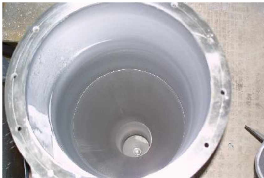
(e) Almost clean cyclone body at ( V1200_{\mu_e 3.0} ).
