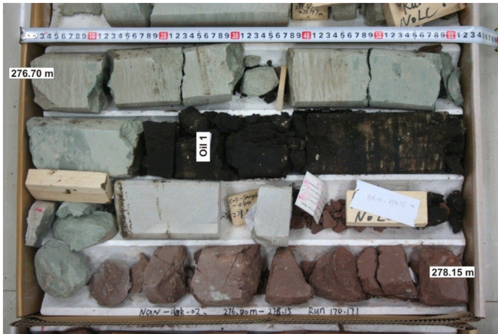
Figure 7: Oil-stained sandstone in the Quantou Formation of borehole NGN-dgk-02.
