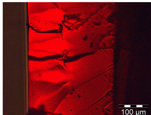
Figure 103: Microscopy image of written waveguide cross sections in silanol terminated polysiloxane cross-linked with 20 wt. % acryloxymethyl trimethoxy silane, 0.05 wt. % butyl-N-DPD
