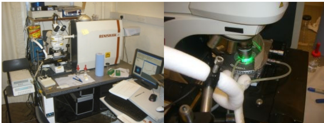
Figure 3.1: Raman spectrometer Renishaw 1000 at King’s College London (left). During measurements the temperature was controlled by the Linkam THS 600 cooling stage (right).
