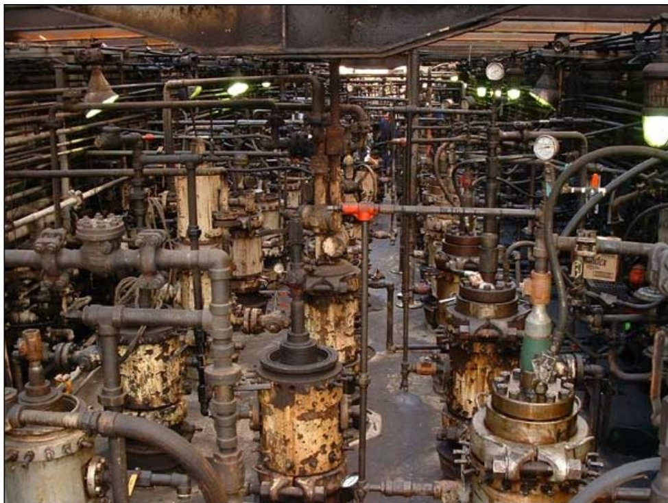
These are actual wellheads for an urban drill site. Most of the wells in this picture are Hydraulic Rod Pumps.
