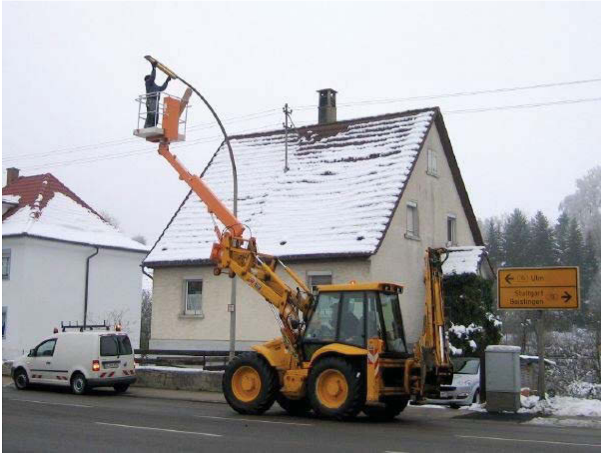
Figure 173: Additional equipment, lifting platform mounted on the loader, exemplary (cp. Kran & Hebetchnik 2007 12 )
