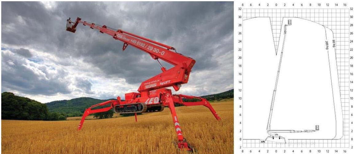
Figure 172: Additional equipment, chain mounted lifting platform (cp GL Arbeitsbühnen Verleih 11 )
