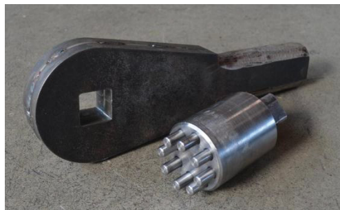
Figure 32: Cone Wrench to hold Modified Nut while tightening Pin
