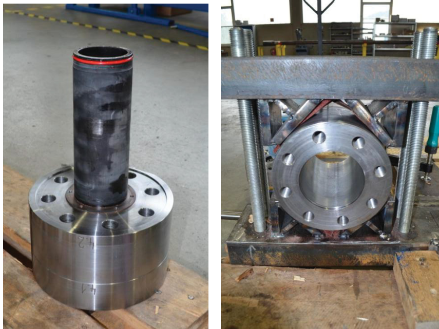
Figure 55: Oil-free Inner Components after Testing
