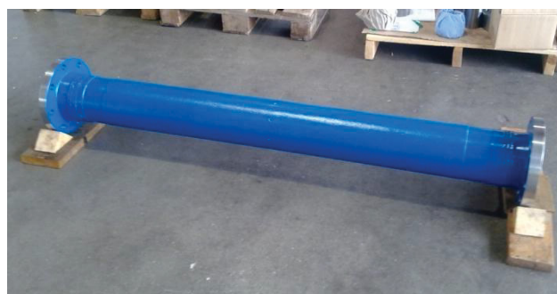
Figure 20: Main Pipe with Flanges
