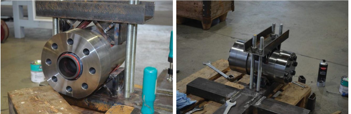
Figure 52: Mounting O-rings and End Plates
