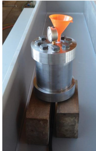
Figure 38: Filling of the Test Cell in upright Position
