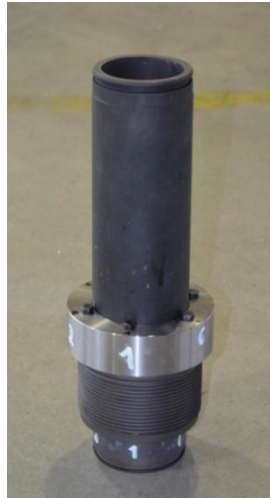
Figure 49: Protective Bushing screwed in Liner Nut (hand tight) with Ring of Mounting Tool
