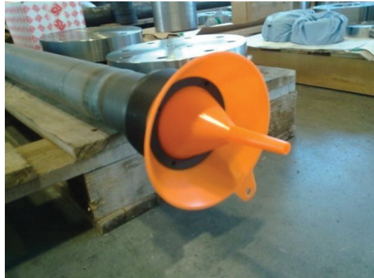
Figure 43: Funnels for Filling the Liner&Sealing Test Bed
