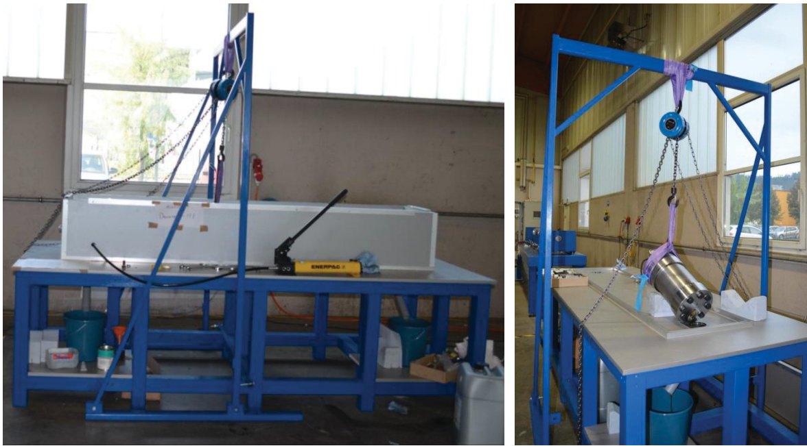
Figure 31: Using the Bench and the Hoisting Equipment (right for oil discharge)
