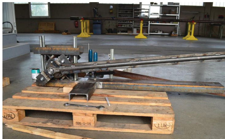
Figure 37: Testbed in Fixation Prism with Axial Fixation ready to apply Torque
