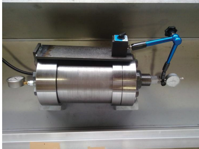
Figure 47: Test Setup for the Extensometer
