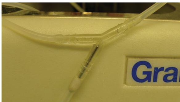
Figure 33: Y-fitting with narrowing at the inlet
