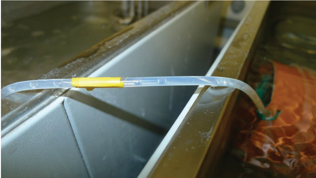
Figure 32: Slug flow in crystallization tube
