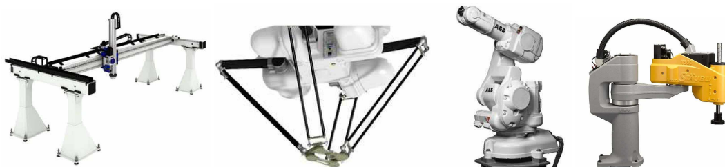
Figure 3: Gantry robot 16 , delta robot 17 , articulated robot 18 and SCARA 19 (from left to right)
