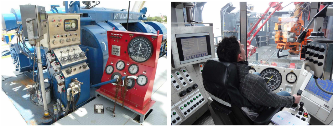
Figure 19: Driller's console next to the hoisting drum (left) and modern driller's cabin (right)
