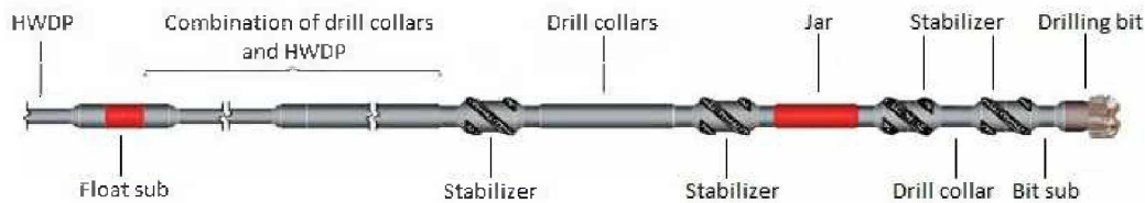
Figure 34: Example for a BHA setup 68
