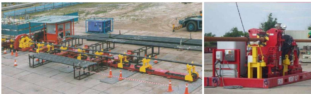
Figure 41: Offline assembling of BHA (left), mobile bucking unit (right)
