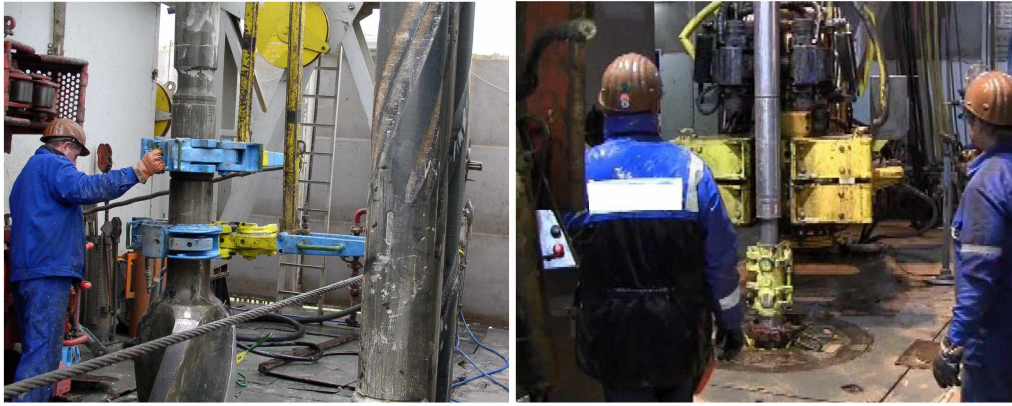
Figure 23: Manual tongs (left) and iron roughneck (right)
