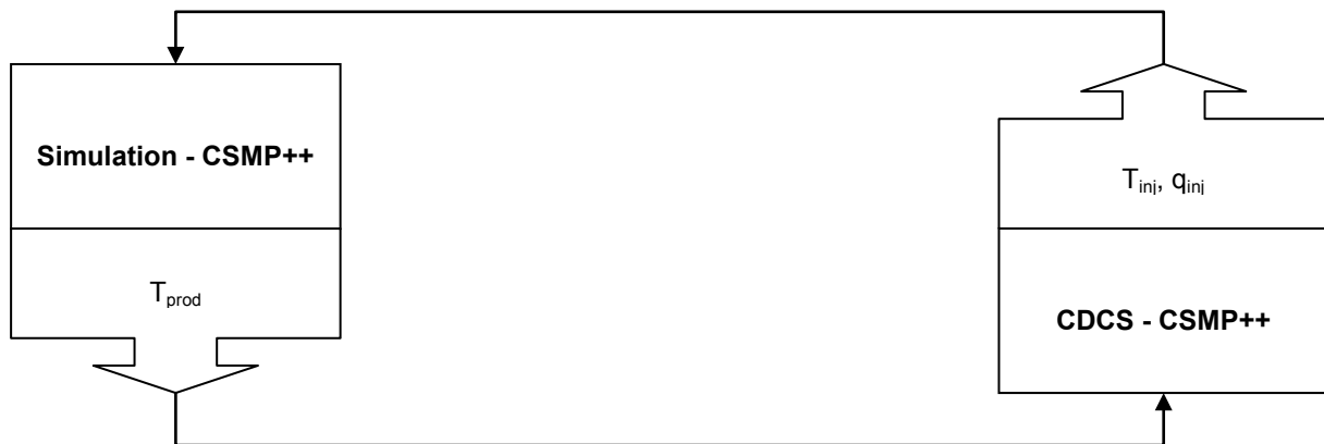
Fig. 3.3: Communication between the thermal simulator and the CDCS. The simulator receives the injection temperature and rate for the next time iteration and the CDCS obtains the temperature at the production well.
