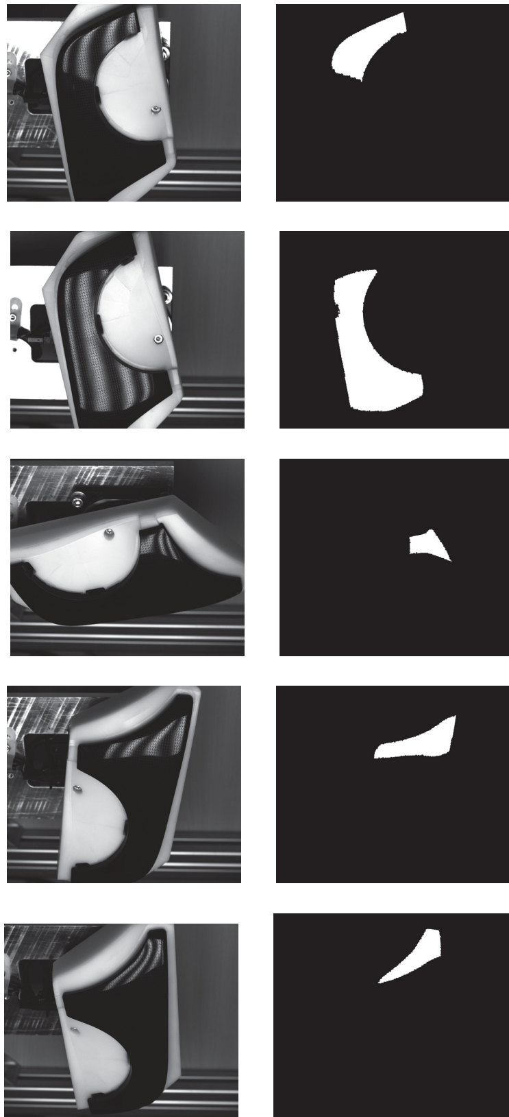
Figure 3.6: Left column: Example of measurement image for each position. Right column: Black and white maps marking the inspected surface areas which are inspected in the respective deflectometric measurement.
