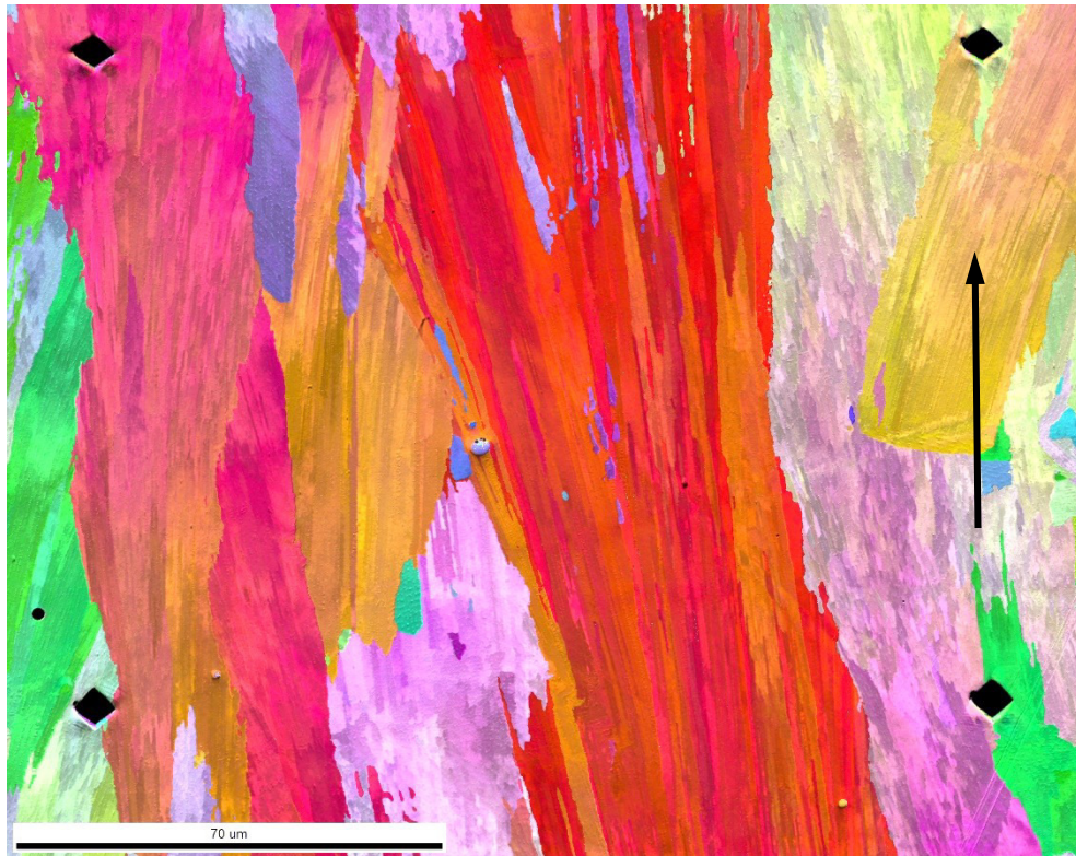
Figure 41: Overlay of an EBSD image with the inverse pole map of the SLM structure. If the energy input is high enough, large grains will grow epitaxially over several deposited layers. The building direction is indicated by an arrow.
