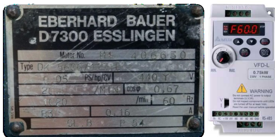
Figure 70: Specifications of the motor for the rotary valve and the motor drive regulator Delta CFD-L
