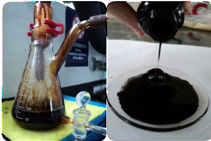
Figure 72: Erlenmeyer flask to collect the oil of the pyrolysis process (on the left) and the pyrolysis oil (on the right sight)
