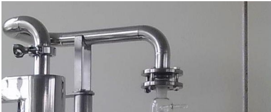
Figure 88: Connecting tube between cyclone and glass condenser
