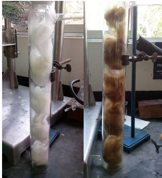
Figure 59: Control filter of the pyrolysis plant: new installed filter (on the left); filter after the experiment (on the right)
