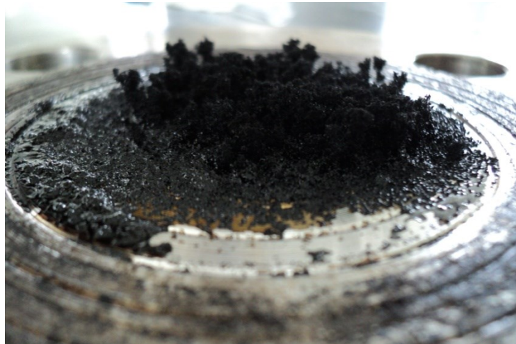
Figure 87: Deposits formation on the reactor cover blade
