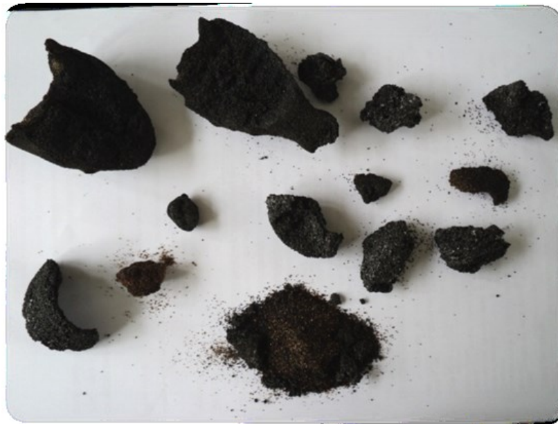
Figure 78: Residues that plugged the reactor when using cooked rice as raw material feedstock.
