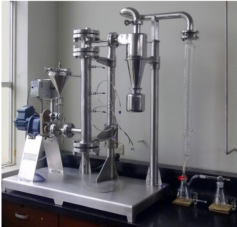
Figure 63: Assembled PUCP-pyrolysis plant without heating, electric installations and isolation.
