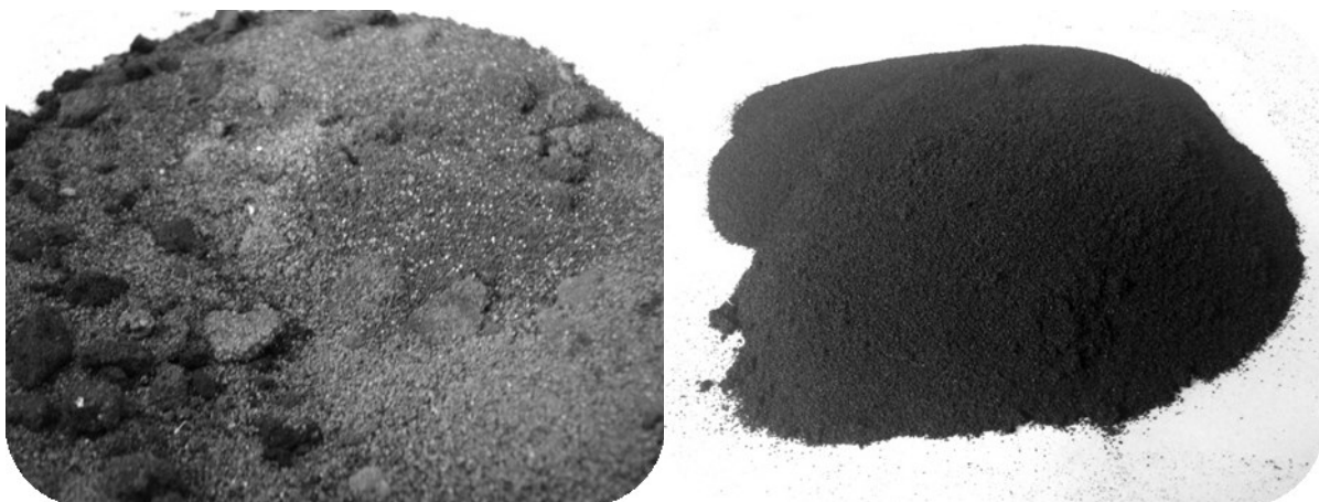
Figure 76: Char from the reactor mixed with quartz sand (on the left) and char collected in the collecting bin (on the right)
