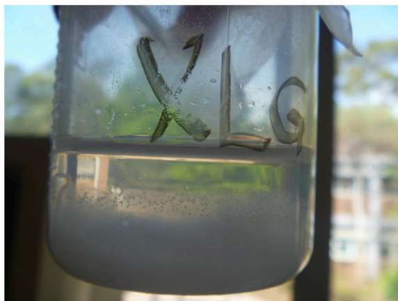
Figure 4.1: Clay-water mixture: After several weeks without stirring clay is not fully dispersed in water.
