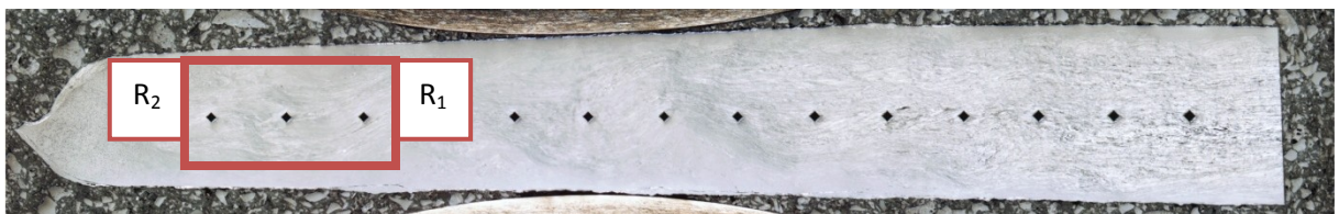
Fig. 4.5: Area for further SEM investigations on a heat treated two step sample.
