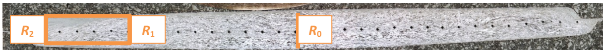
Fig. 4.3: Light microscopy picture of the whole radial sector of a one step HPT sample. The centre position ( R_0 = 0.0 mm) and an area of interest (from R_1 = 2.5 mm to R_2 = 3.5 mm) are pointed out.
