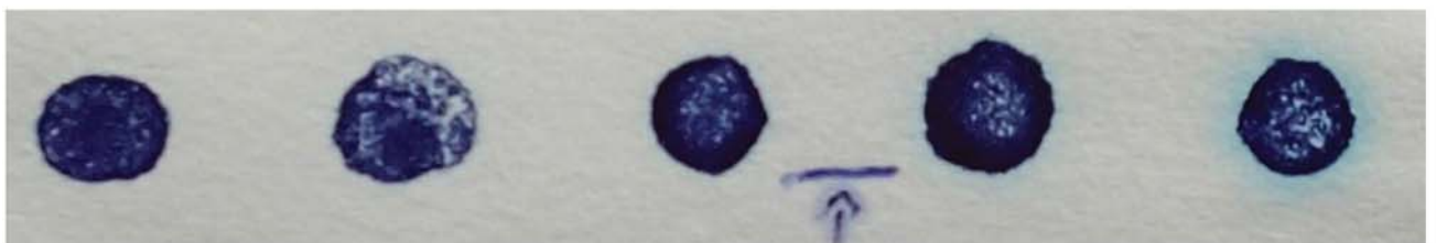
Fig. 8: Methylene-blue Adsorption Filter Paper, Sample Zelenika (m = 0,4999 g, H 2 O = 8,95%, Arrow at 22,5 ml)
