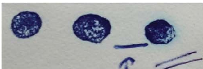
Fig. 9: MB Adsorption Filter Paper, Sample Ralitsa (m = 0,5002 g, H 2 O = 10,65%, Arrow at 19,5 ml)
