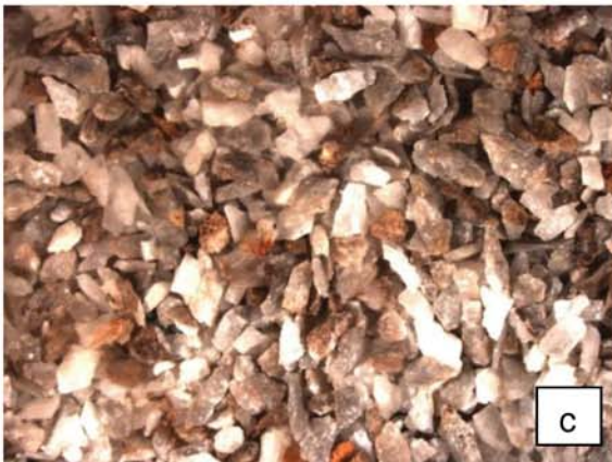
Fig. 48: Electrostatic Separation Products, Barite, Binocular Pictures, k=0.71-1mm: a = CP. b = IP. c = WP
