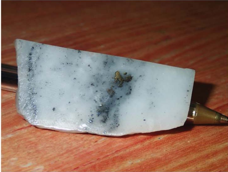
Fig. 15: Polished Section of Barite with Sulfides
