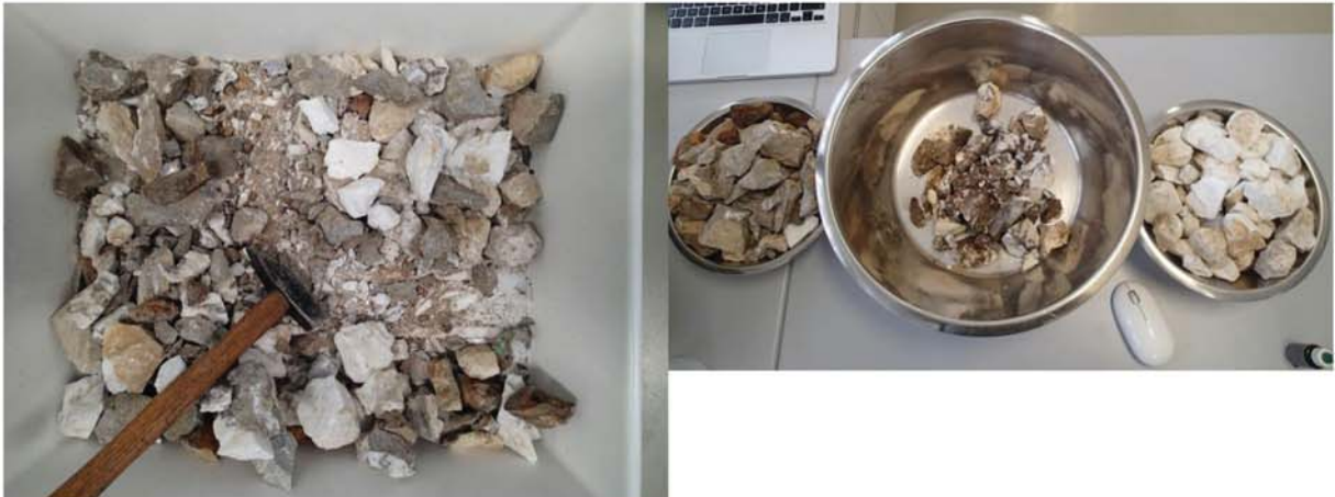
Fig. 30: Subsample of One Quarter of the Aggregate Sample (left); Optical Sorting into 3 Products (right)
