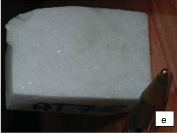
Fig. 18: a : AT-7A, Barite with Quartz; b: AT-7B, Barite with Quartz; c: AT-7C, Barite with Sulfides; d: AT-7D, Barite with Sulfides; e: AT-7E, Barite, with greenish Impurities
