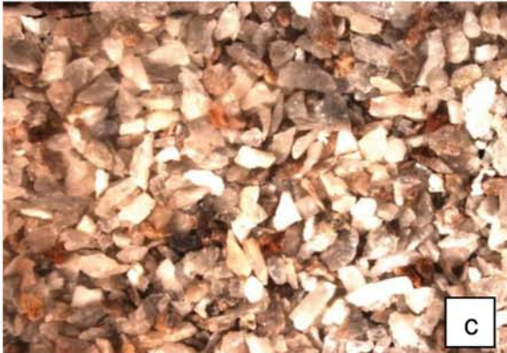
Fig. 49: Electrostatic Separation Products, Barite, Binocular Pictures, k=0.5-0.71mm: a = CP, b = IP, c = WP
