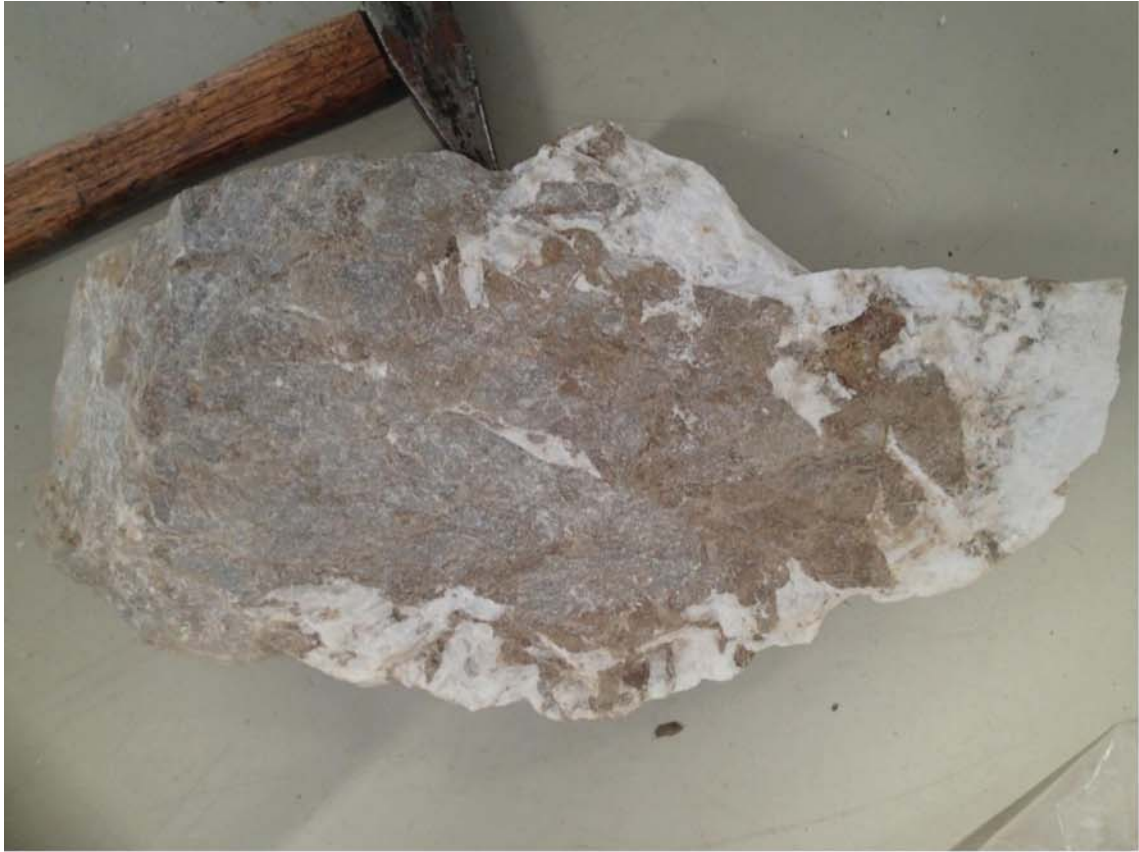
Fig. 20: AT-1K, Barite intergrown with Dolomite
