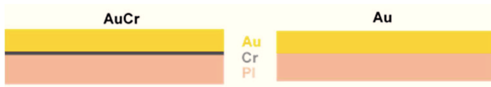
Figure 11: Schematics of the investigated film-substrate systems, AuCr : 50 nm Au film sputter deposited onto a 50 \mu\text{m} polyimide substrate. A 10 nm Cr interlayer is used to improve adhesion; Au : 50 nm Au film sputter deposited onto a 50 \mu\text{m} polyimide substrate, no adhesion layer.
