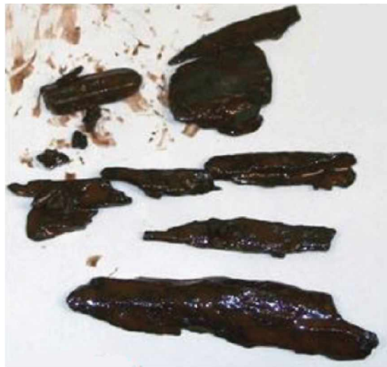
Figure 34: Splintered cavings (Kumar et al. 2012)
