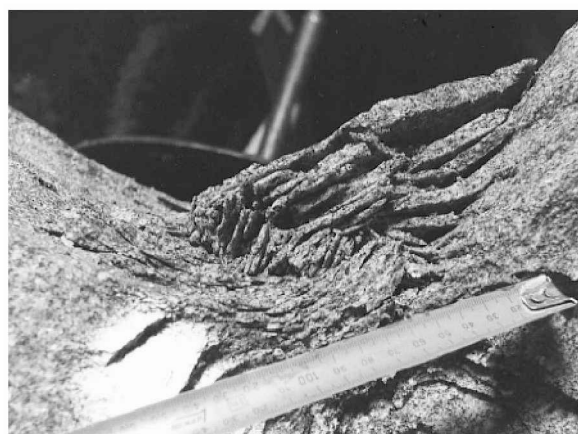
Figure 23: Brittle wellbore behavior (Batchelor & Marks 2010)
