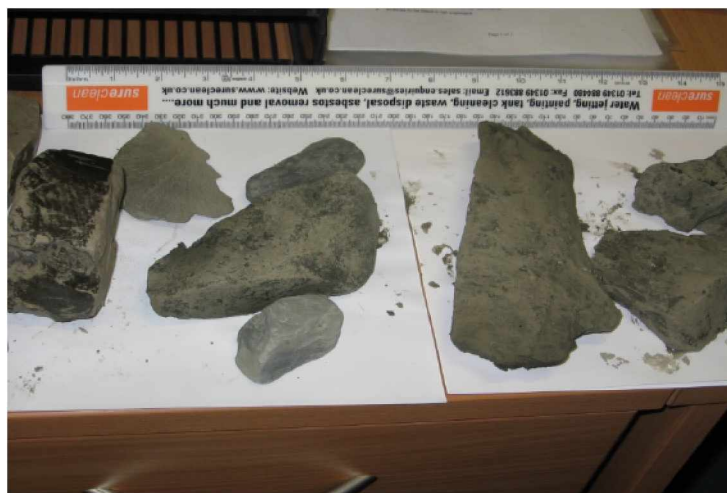
Figure 35: Larger angular cavings (Batchelor & Marks 2010)
