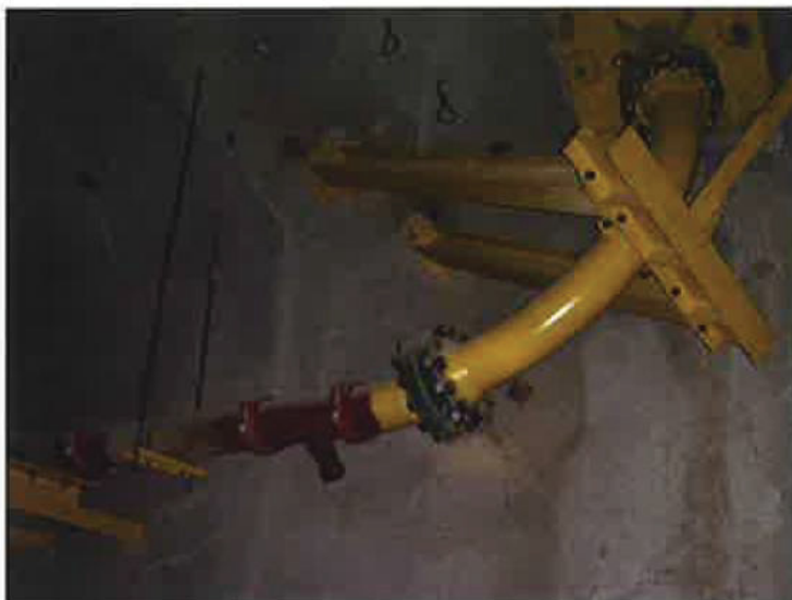
Figure 25: Sacrificial part of a pipeline system 17 p.184
