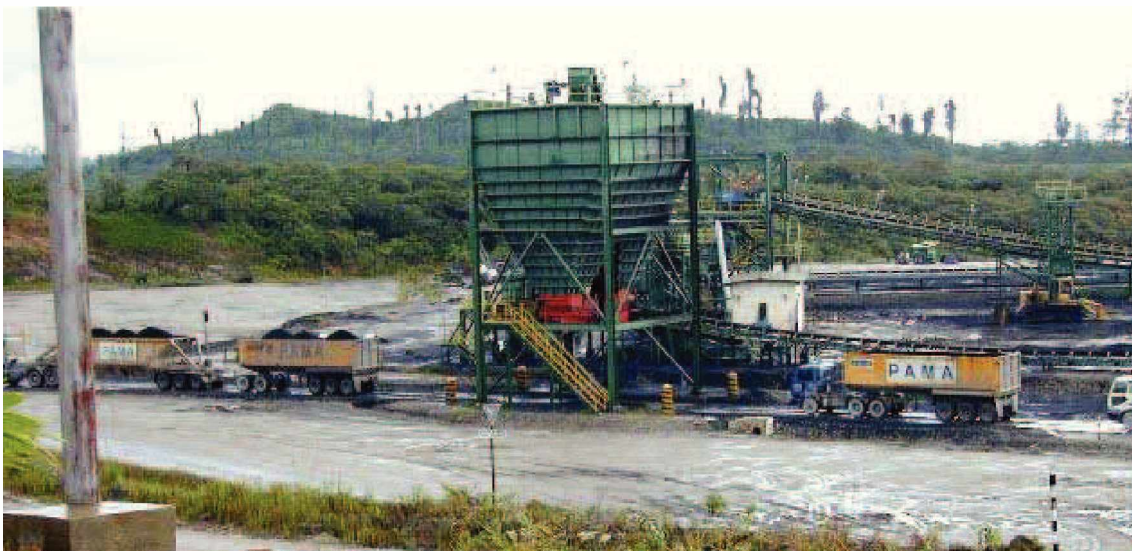
Fig. 3–30: Haulage trucks transport the material out of the mine to the crushing unit
