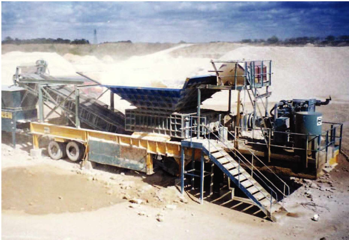
Fig. 3-11: Mobile crusher with pneumatic tyres
