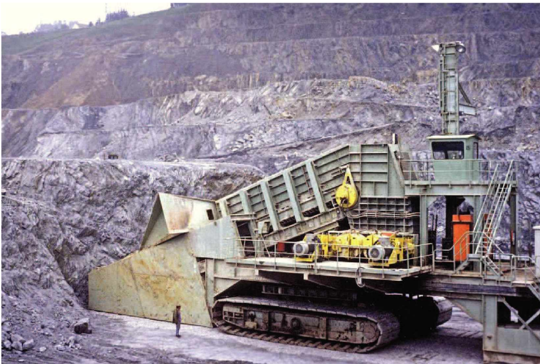
Fig. 3-10: MMD Semi-mobile Sizer at Lignitos de Meirama/Spain
