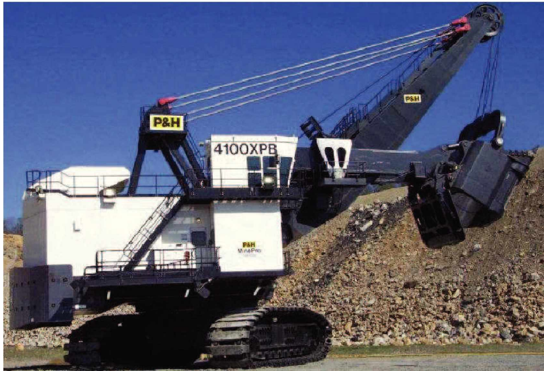
Fig. 5-10: Rope shovel excavator P&H 4100 XPB
