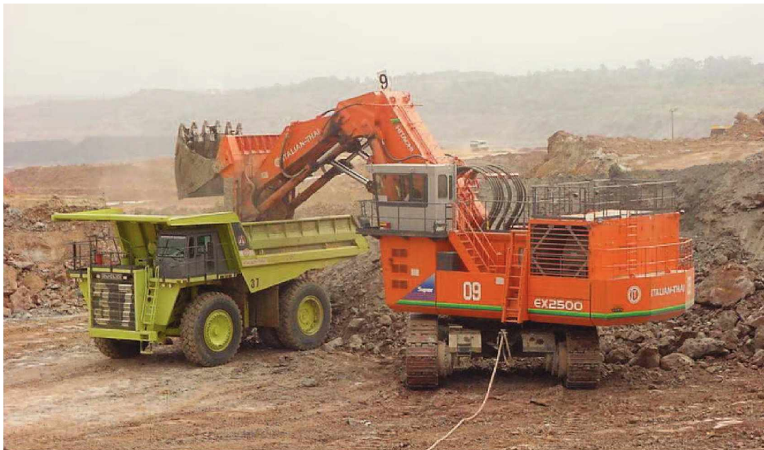
Fig. 3-35: Hydraulic excavator Hitachi EX2500E loading a truck Euclid-Hitachi EH1700
