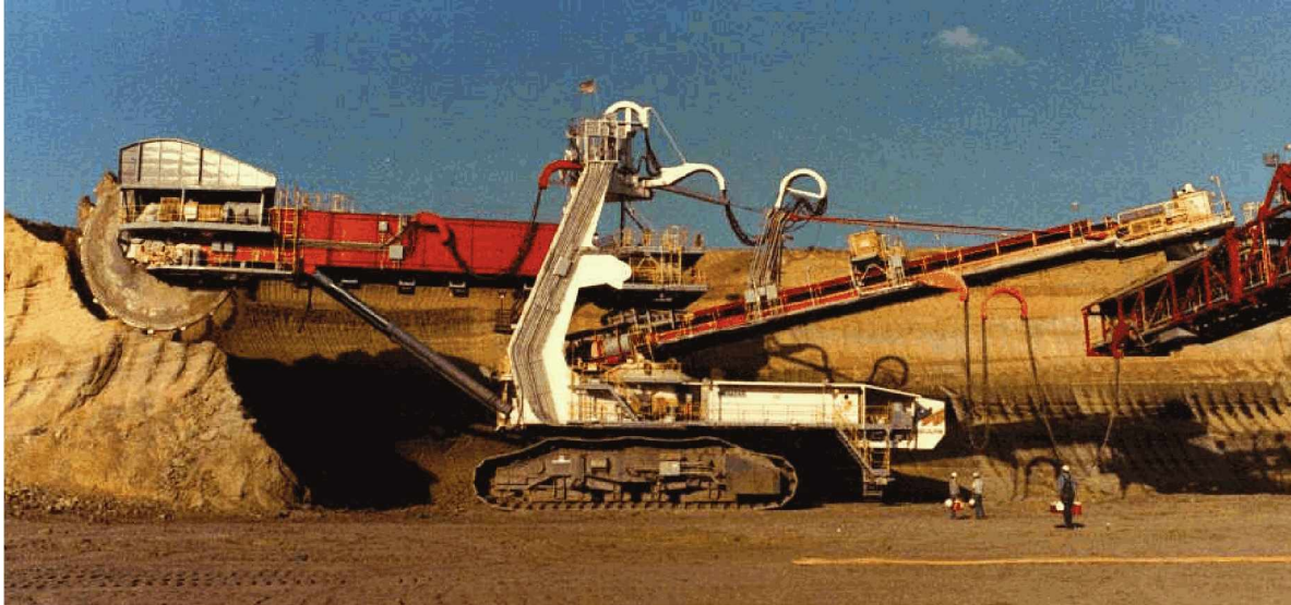
Fig. 3-5: Bucket wheel excavator Type VABE 1500 in Monticello/USA
