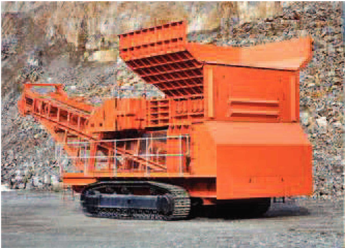
Fig. 3-12: Mobile crusher with crawlers
