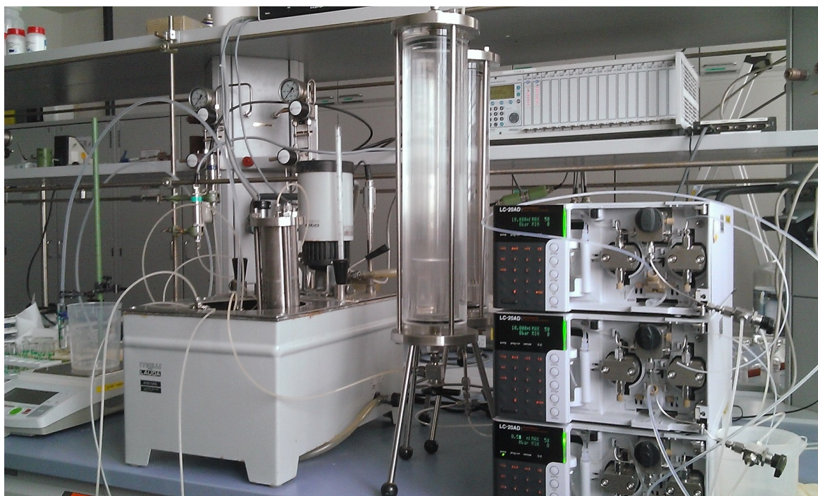
Figure 18: Core flooding equipment including HPLC pumps, hydraulic containers, a water bath, scales and the core.
