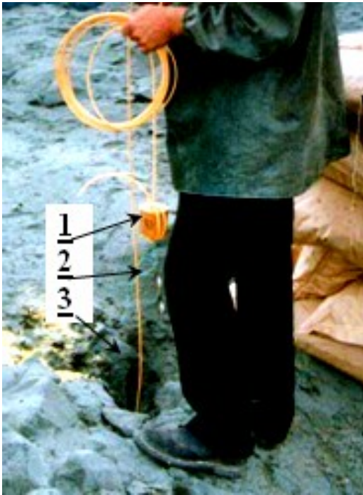
Fig. 2.11 Setting the turbulator of detonation products.
