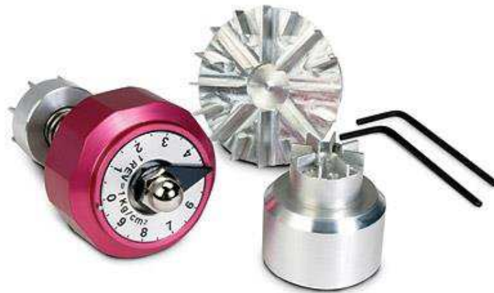
Figure 5-9: Torvane or pocket shear vane, the photo is taken from [23]
