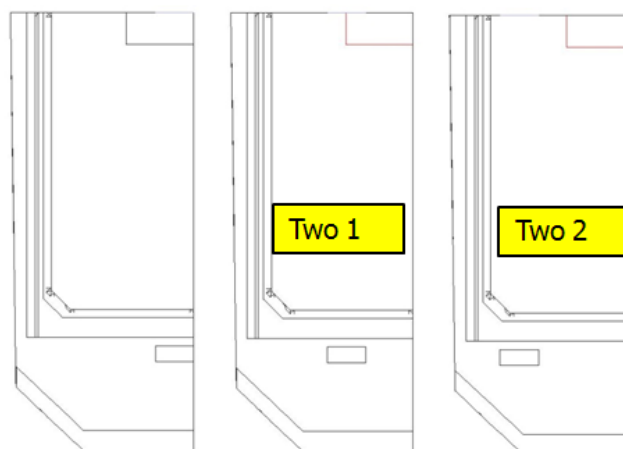
Figure 93: Inlet designs for the multi inlet design study: The standard case was compared to two cases with off center inlet positioning (Two 1 and Two 2)
