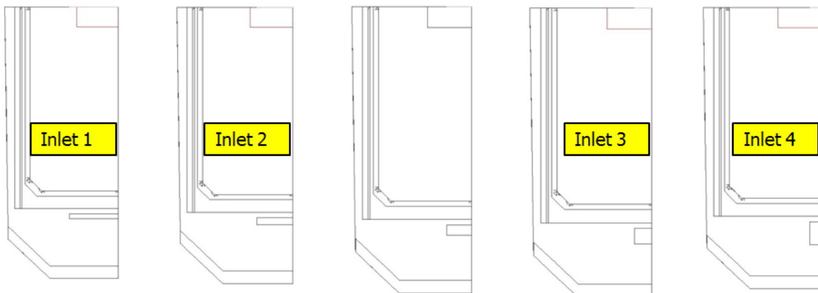
Figure 87: Inlet designs for the variation of inlet shape studies: The standard case was compared to two wide inlet cases (Inlet 1, Inlet 2) and two narrow inlet cases (Inlet 3 and Inlet 4)
