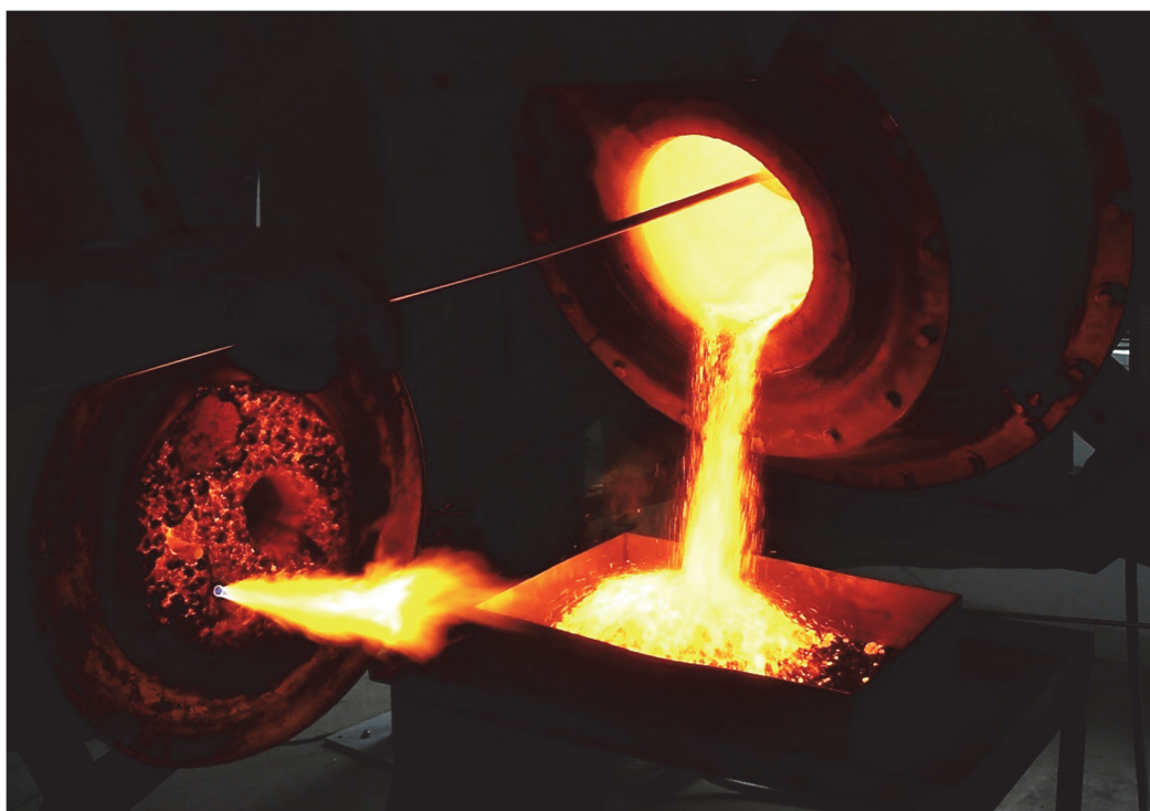
Figure 6-11: Tapping of clinkered material from the TBRC
