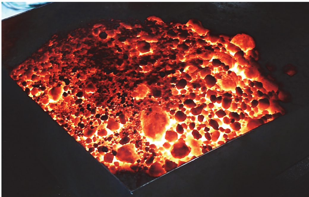
Figure 6-12: Hot clinkered material soon after tapping
