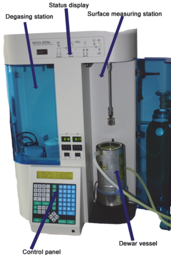
Figure 2-6: “Quantachrome Instruments NOVA 2000e” for the measurement of the specific surface area and pore size distribution
