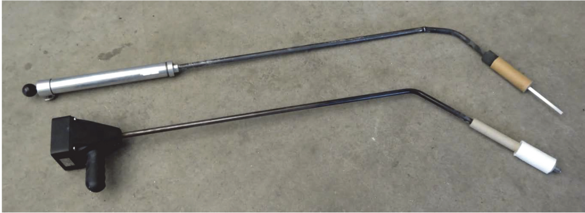
Figure 4-14: Vacuum sample taker (top) and temperature measurement lance (bottom), both with single use attachment for sampling and temperature measurement, respectively
