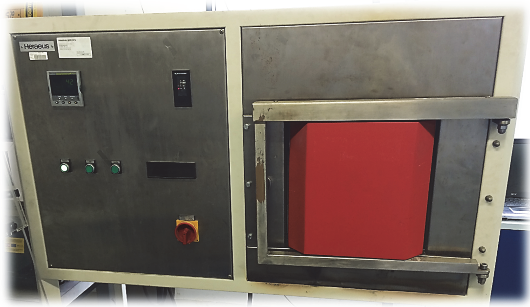
Figure 4-8: High-temperature heat resistance furnace “Heraeus K 1750”
