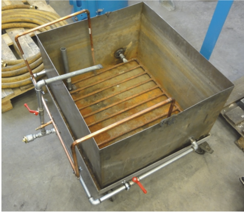
Figure 4-15: Water basin optimized for the granulation of liquid iron
