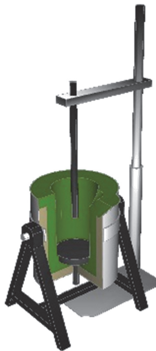
Figure 6-13: Schematic drawing of the applied submerged arc furnace [163]
