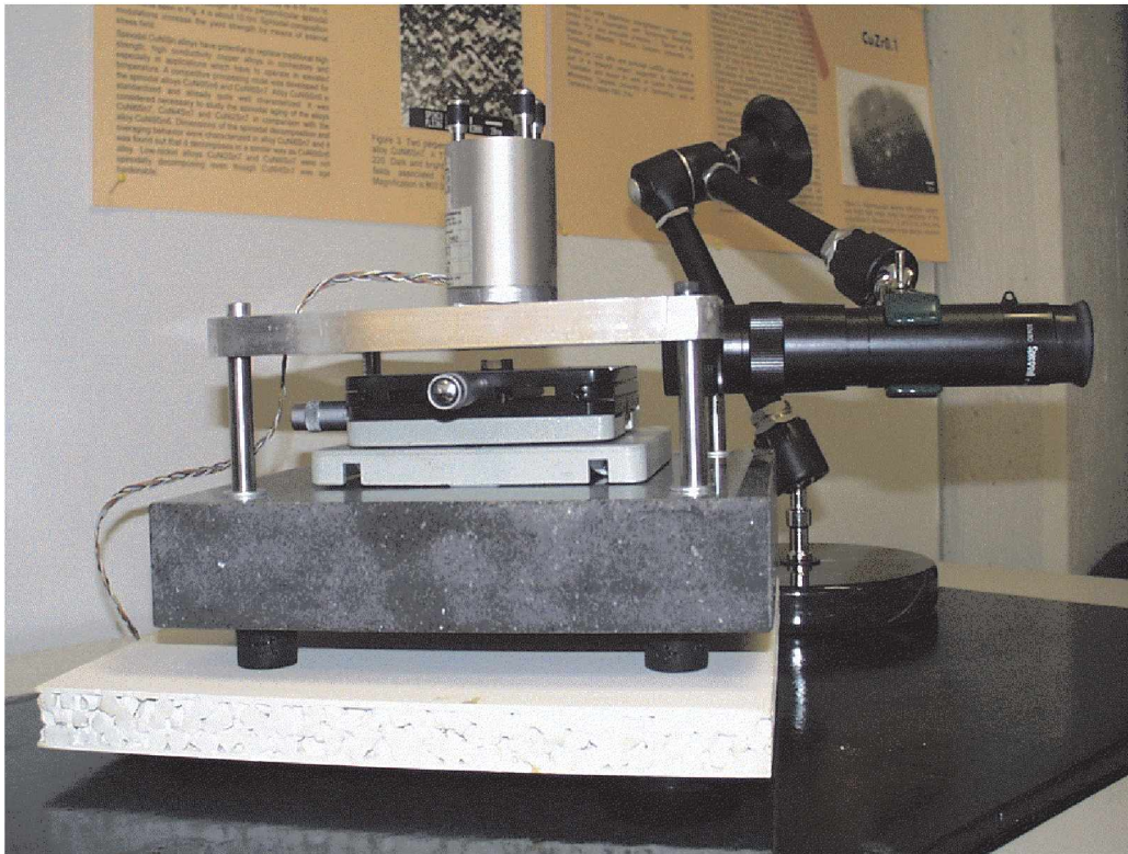
Figure 6-3 Final holder with improved damping.
