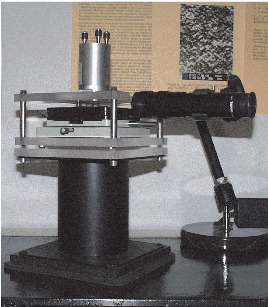
Figure 6-1 First design for the StandAlone (Sample) Holder.
