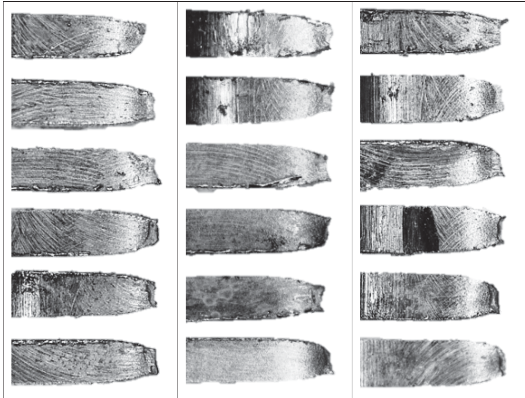
Figure B.11.: Fracture surfaces of micro-samples machined from tubes A (a), B (b) and C (c) after tensile experiments. The top-bottom sequence corresponds to outer-inner sample position in tube wall.
