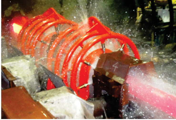
Figure 1.2.: Cooling devices for accelerated tube surface cooling.
