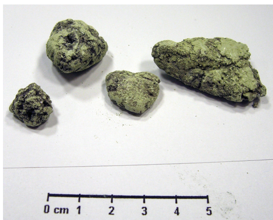
(e) Sintered chips from the container at the end of the kiln "D-Mo-Ta 9"
