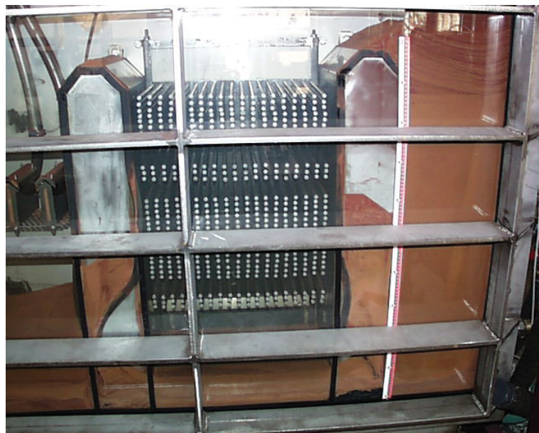
Photo 4.3-1 Installation of a heat exchanging bundle in the second heating chamber of the cold model's FHE
