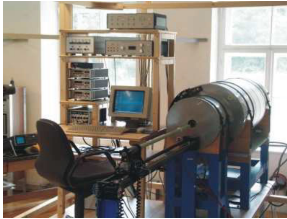
Figure 2.7: 2G DC-SQUID magnetometer, paleomagnetic laboratory Gams, University of Leoben, Austria
