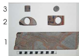
Figure 3.4: Sample 654 illustrates the three preparation steps: 1) halved drill core, 2) ~3cm core slices and 3) plugs with a length of ~20mm and a diameter of 20–25.4mm.
