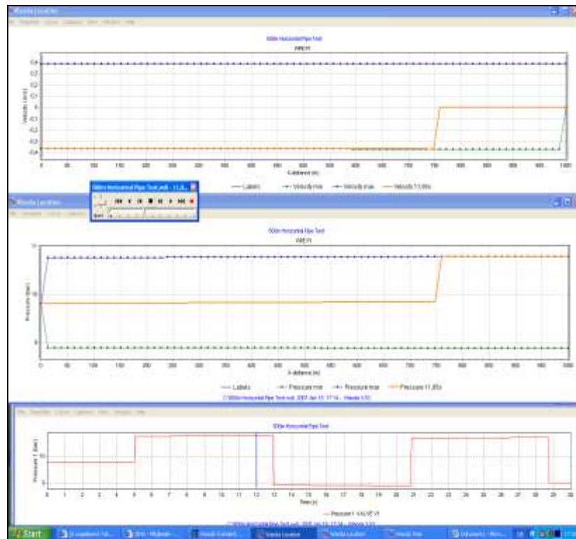
Figure 31: Pressure wave was reflected, fluid exits pipe through the inlet
