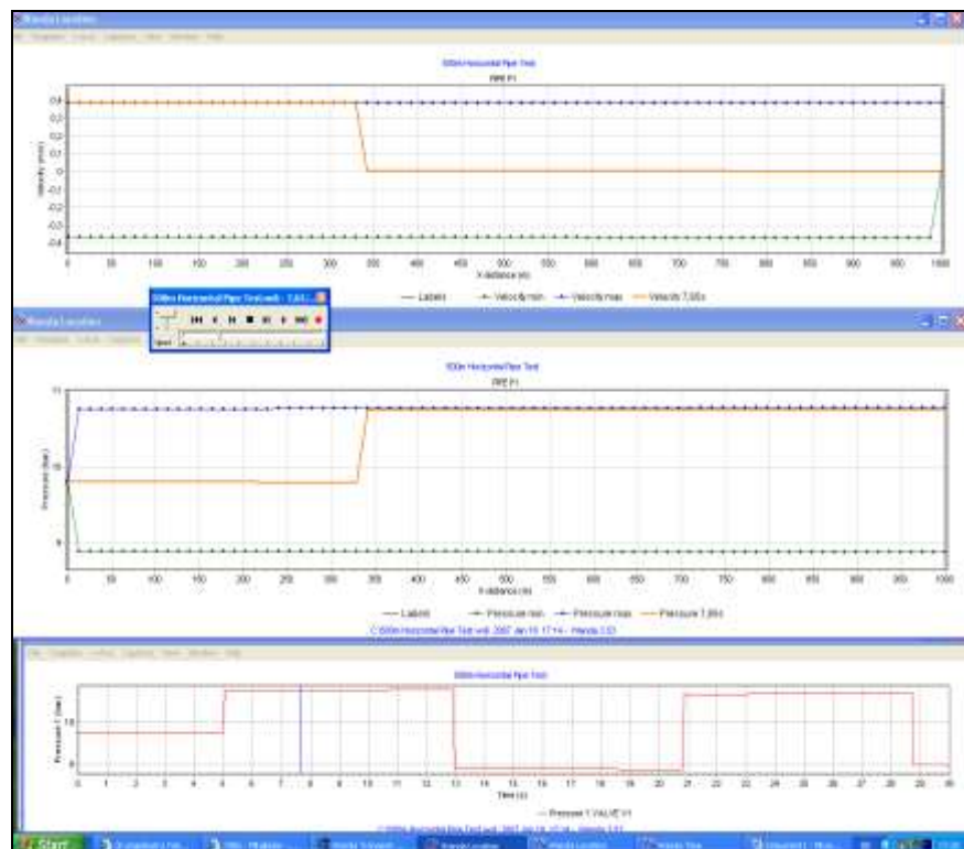
Figure 29: Pressure wave propagates towards the inlet, zero fluid velocity behind the wave front
