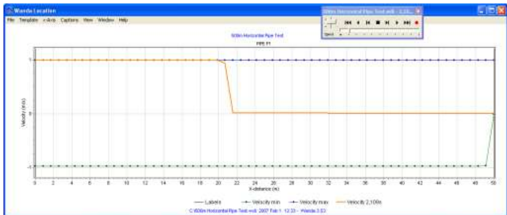
Figure 27: Pressure wave causes change in fluid velocity
