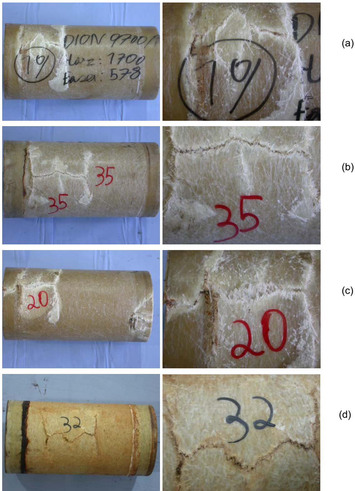
Fig. 4.25: Pictures of fracture pattern from internal pressure test specimens. On the left side a macroscopic and on the right side a detailed picture is shown. Time until failure [h]: (a) 0.17, (b) 0.8, (c) 1.1, (d) 2.
