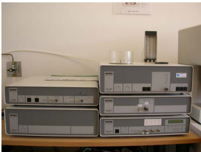
Fig. 3.10: DSC 200 apparatus (4) (Manufacturer: Netzsch / No: DSC 200).
