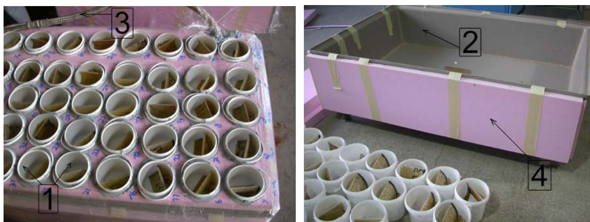
Fig. 3.17: Construction for specimen immersion (Manufacturer: Self-made)
