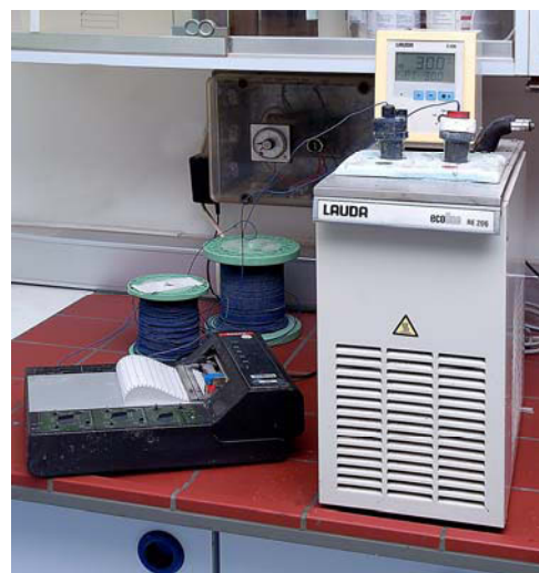
Fig. 3.9: Resin reactivity apparatus (3) (Manufacturer: LAUDA – ECOLINE No: RE 206)
