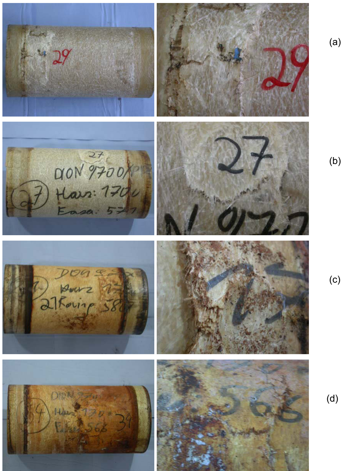
Fig. 7.30: Pictures of fracture pattern from internal pressure test specimens. On the left side a macroscopic and on the right side a detailed picture is shown. Time until failure [h]: (a) 395.7, (b) 478.4, (c) 1114, (d) 2683.9
