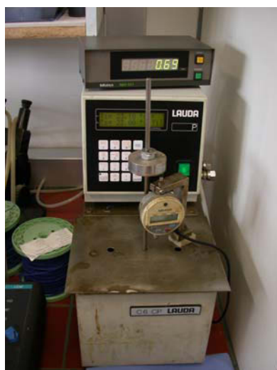
Fig. 3.12: HDT apparatus (Manufacturer: Lauda / C6 CP)
