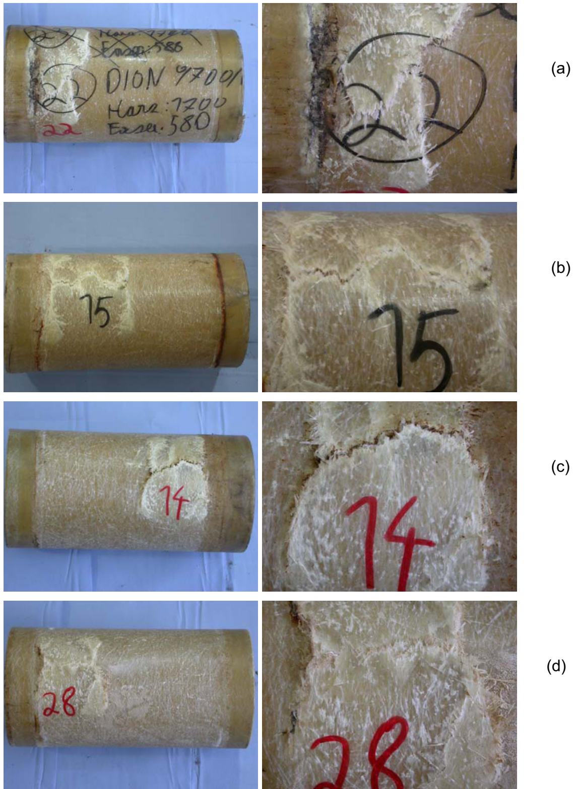
Fig. 7.28: Pictures of fracture pattern from internal pressure test specimens. On the left side a macroscopic and on the right side a detailed picture is shown. Time until failure [h]: (a) 8.5, (b) 16, (c) 41.5, (d) 61.5.
