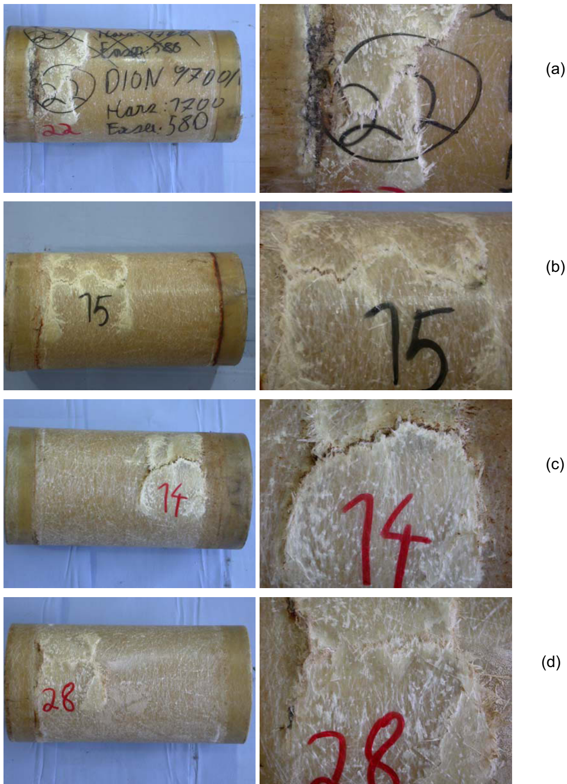
Fig. 4.26: Pictures of fracture pattern from internal pressure test specimens. On the left side a macroscopic and on the right side a detailed picture is shown. Time until failure [h]: (a) 8.5, (b) 16, (c) 41.5, (d) 61.5.
