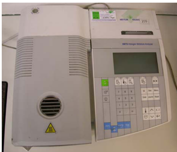
Fig. 3.8: Solid matter content apparatus (2) (Manufacturer: METTLER - TOLEDO No: SNR 1118090365)
