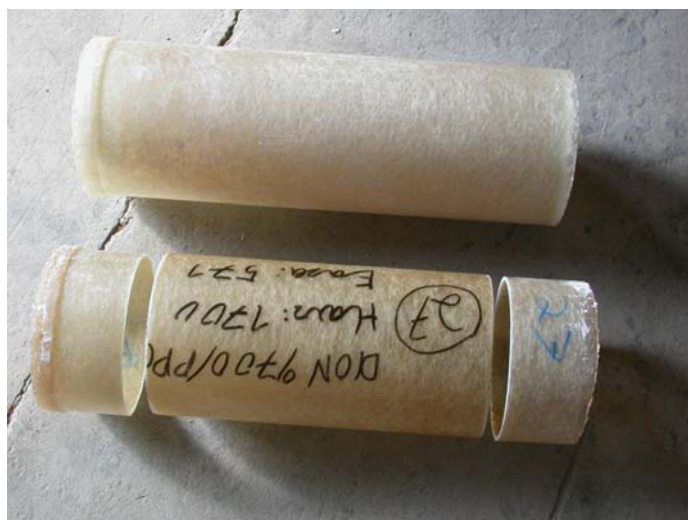
Fig. 3.23: Finished test specimen dry room until they were used for the tests.
