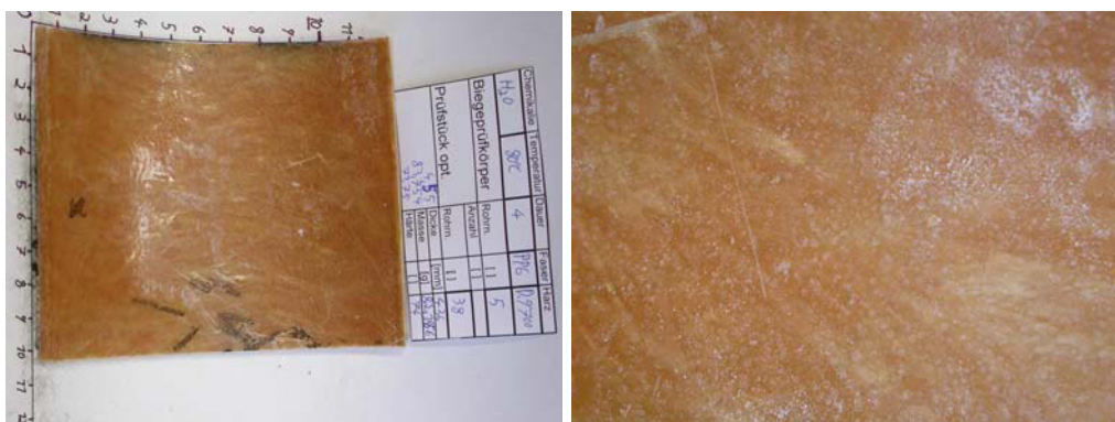
Fig. 7.8: Pictures of specimen for the optical evaluation. The shown specimens were produced with the resin type R1 and fibre F1. The pictures on the left side show the hole specimen, the once on the right side show a close-up view. The specimen on the top of each box show the specimen before immersion, the once downwards show the specimen after its longest immersion (16,18 weeks) (a) NaOH-23°C, (b) Tenside 23°C, (c) Heating-oil 23°C, (d) H 2 SO 4 50°C (e) NaOH 50°C, (f) H 2 O 50°C, (g) H 2 SO 4 80°C, (h) H 2 O 80°C,
