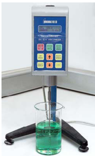
Fig. 3.11: Viscosimeter (5) (Manufacturer: Brookfield / No RVDVII+)
