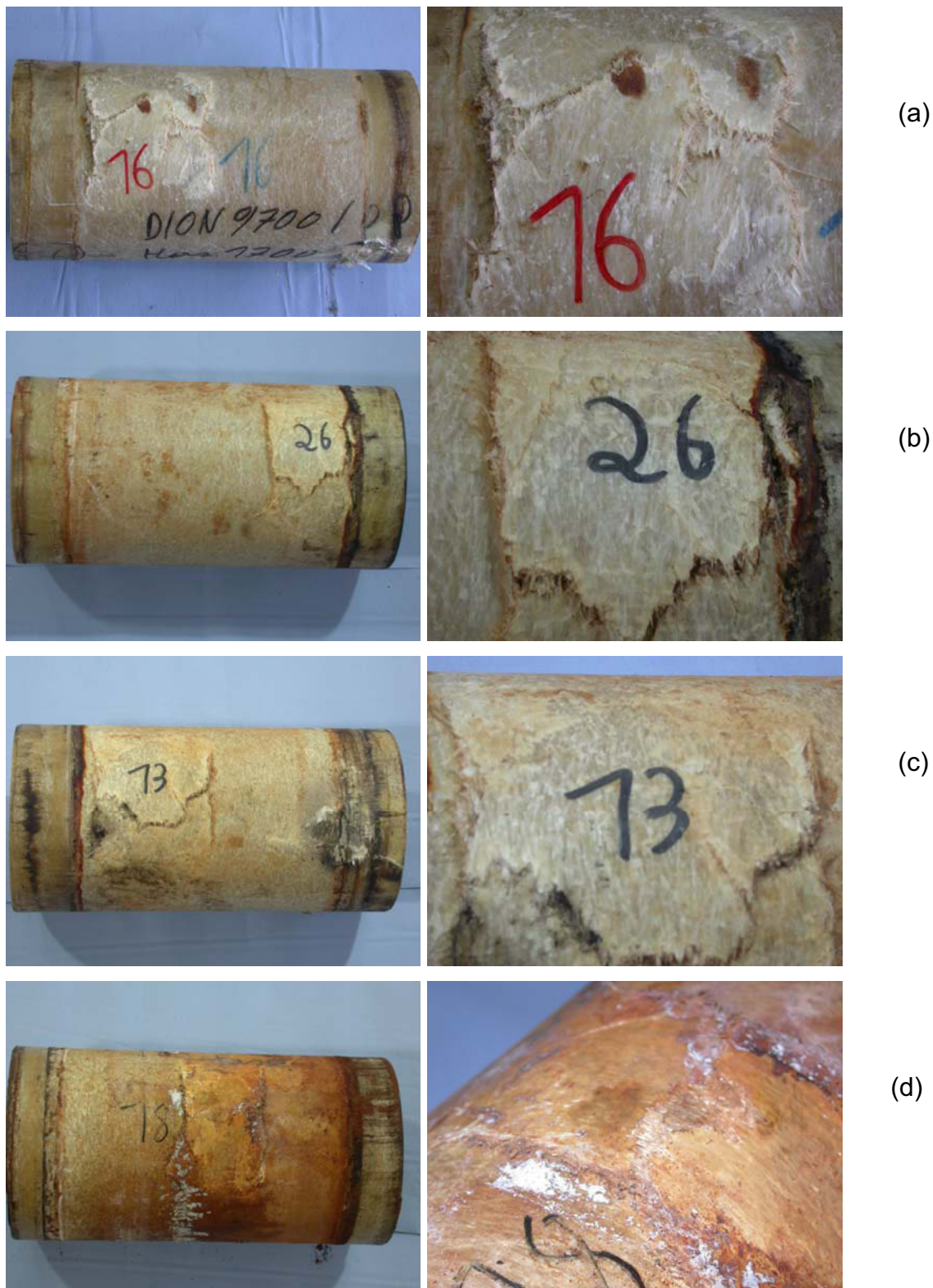
Fig. 4.27: Pictures of fracture pattern from internal pressure test specimens. On the left side a macroscopic and on the right side a detailed picture is shown. Time until failure [h]: (a) 73.3, (b) 84.5, (c) 285.4, (d) 385.6
