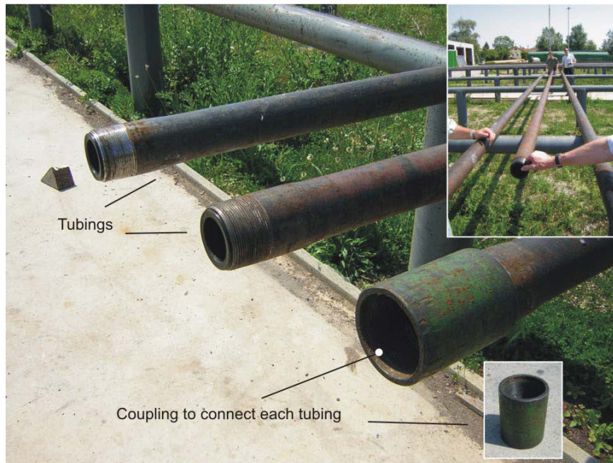
Figure 2.5: Tubings (OMV tube storage Prottes, Austria)
