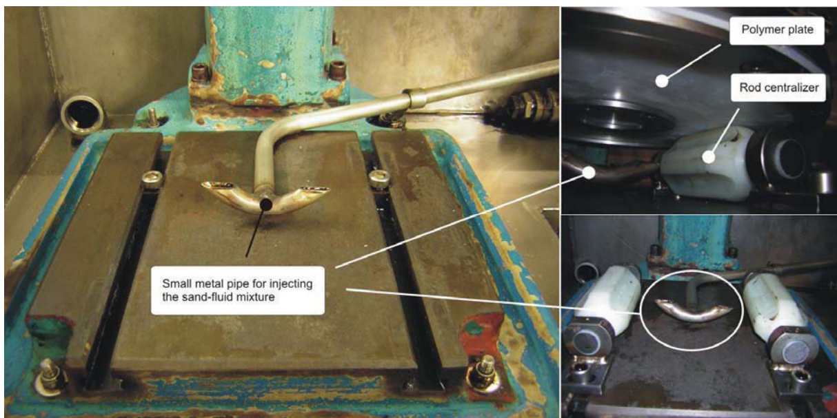
Figure 3.3: Installed metal pipes for injecting sand-fluid mixture.
