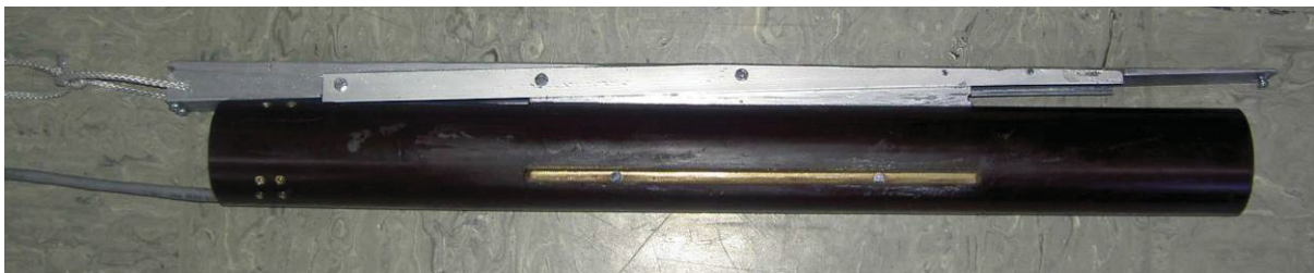
Figure 3.7: Geophone housing with sliding wedge
