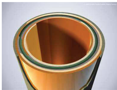
Figure 16: Cross section thought a self expandable casing [26]
