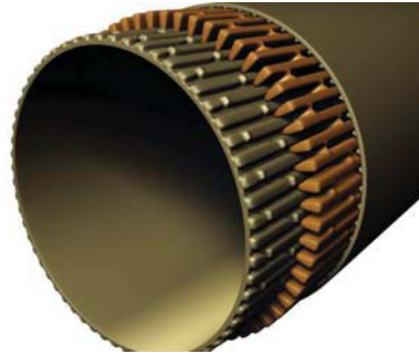
Figure 15: Structure of the self expandable casing [26]
