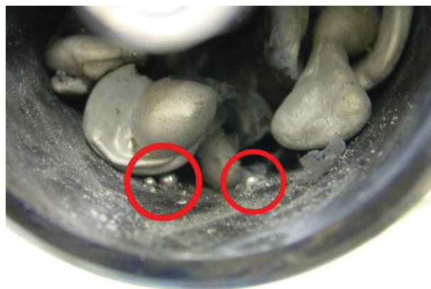
Fig. 4.14: Metallic tin spheres formed in the molybdenum reactor during deposition VI
