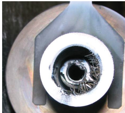
Fig. 4.6: Needle like \text{Cr}_2\text{O}_3 on reactor cap
