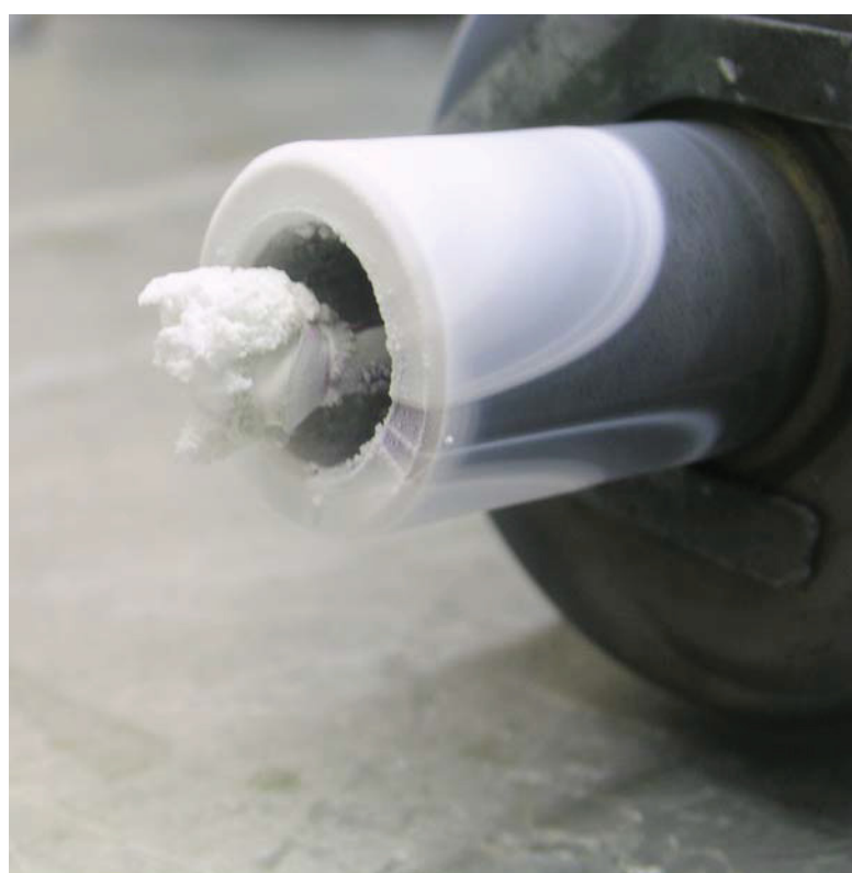
Fig. 4.27: Tin oxide formed on the reactor cap
