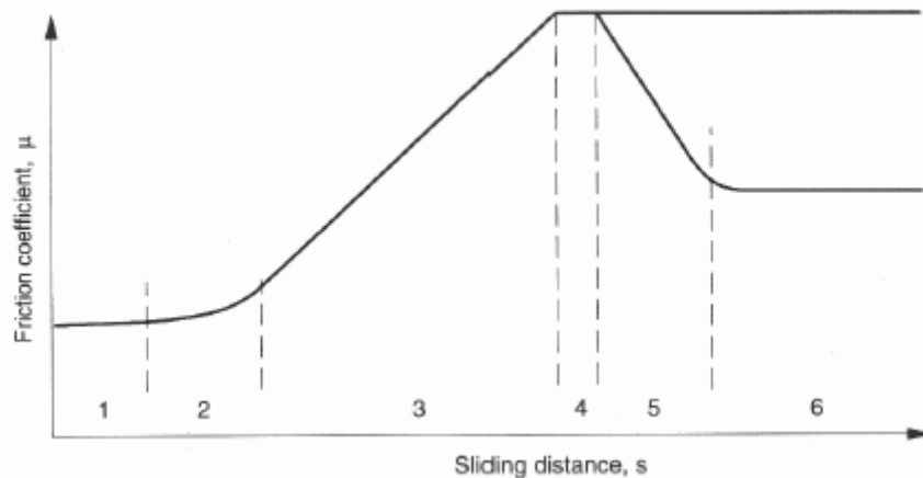
Fig. 2.12 Stages of friction mechanisms vs. sliding distance in sliding steel contacts [35].
