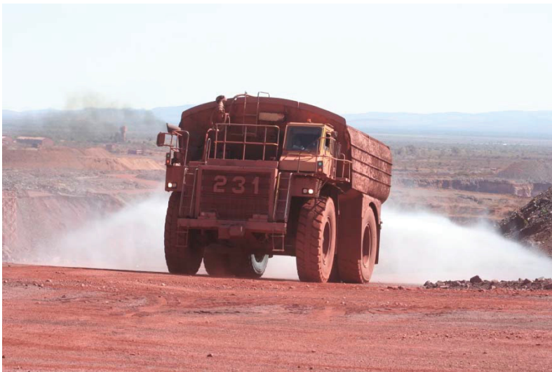
P 36: CAT 777C water-truck (#231) spraying at Bruce stock pile
