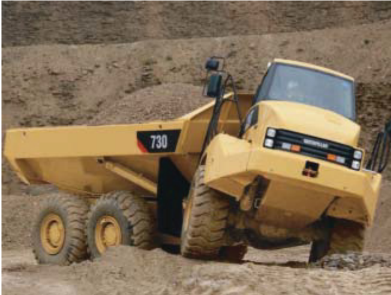
P 42: Demonstration of the turn ability of an articulated dump-truck (Caterpillar, 1998, 2007)
