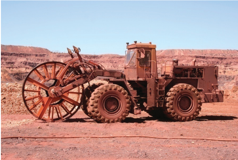
P 52: CAT 834B cable-handler (#024-06) in GR80
