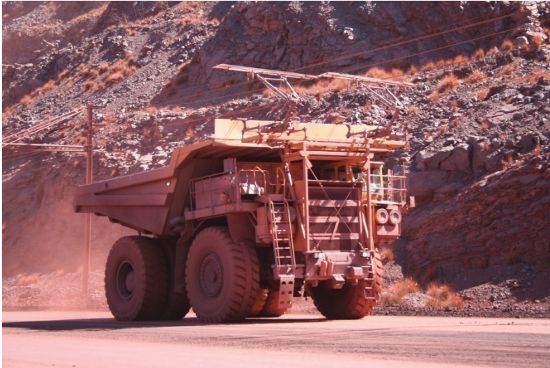
P 57: Lectra Haul (Unitrig) MK36 (#207) on pantograph line in GR35
