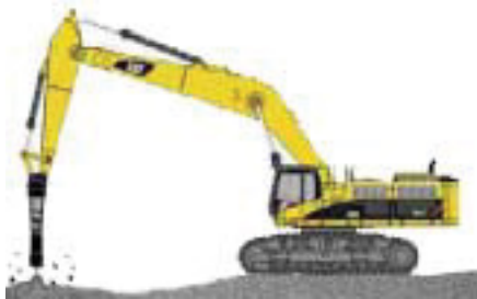
P 49: CAT 385L equipped with a hydraulic hammer (Caterpillar, 1998, 2007)
