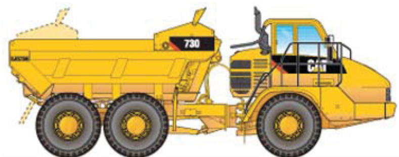
P 44: CAT 730 with a ejector bucket (Caterpillar, 1998, 2007)
