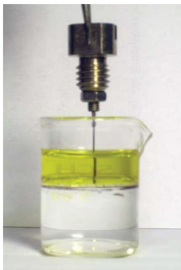
Fig. 18: In the two-step process the electrolyte (yellow) is floating on top of an inert fluid (transparent). The sample is moved up and down in the electrolyte to form a necked region.
