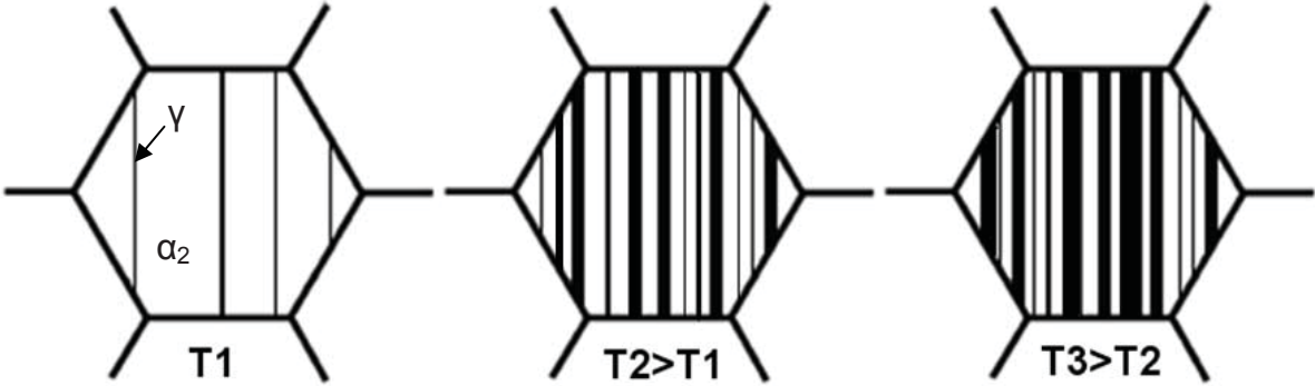
Fig. 57: Model of lamellar colony formation in TNM-B1. After the first heat treatment few fine \gamma -lamellae can be found in the \alpha_2 -grains. During the second heat treatment more \gamma -lamellae nucleate. The interlamellar spacing does not change considerably for higher temperatures in the second heat treatment. The only difference between T_2 and T_3 is the higher volume fraction of \gamma at T_3 .
