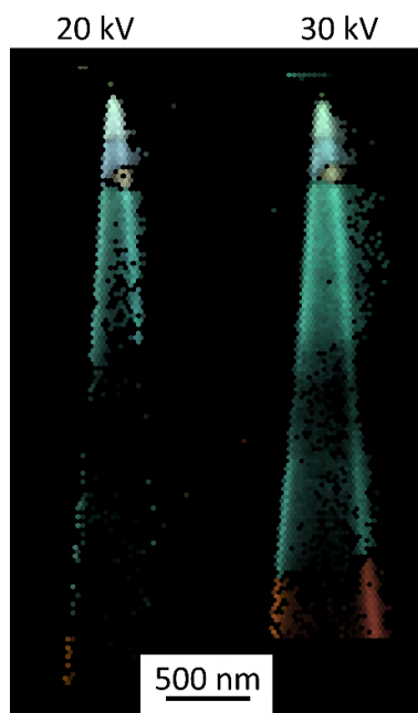
Fig. 5: IQ overlaid with IPF maps of an APT specimen of the as-deformed stage analyzed with 20 kV and 30 kV at a specimen surface tilt of -40^\circ . In the first 500 nm of the molybdenum tip, three low-angle boundaries are visible. At \sim 2.5 \mu\text{m} below the apex a high-angle boundary is present in the specimen. For the IPF coloring inset which indicates the crystal direction perpendicular to the specimen surface please refer to Fig. 2.
