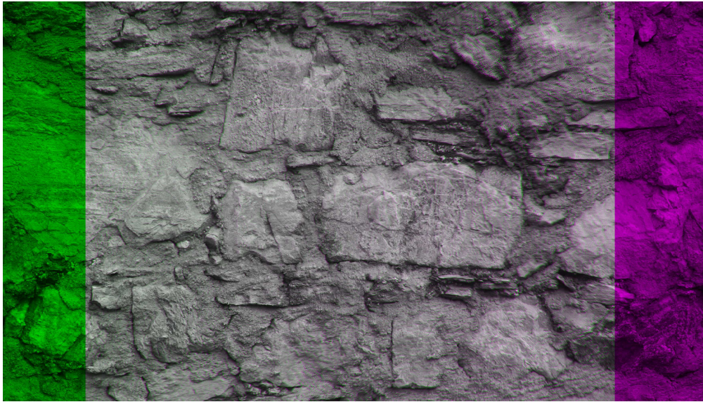
Figure 2.4: Overlay of the registered images according to the result of the phase correlation.
