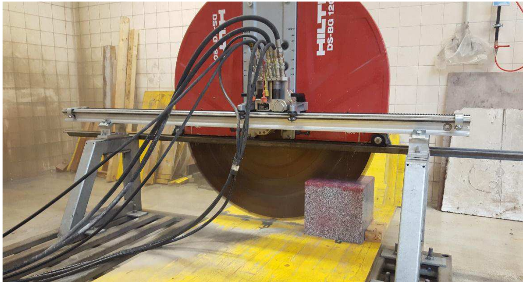
Figure 37: Cutting the cube A along the radiation spots.
