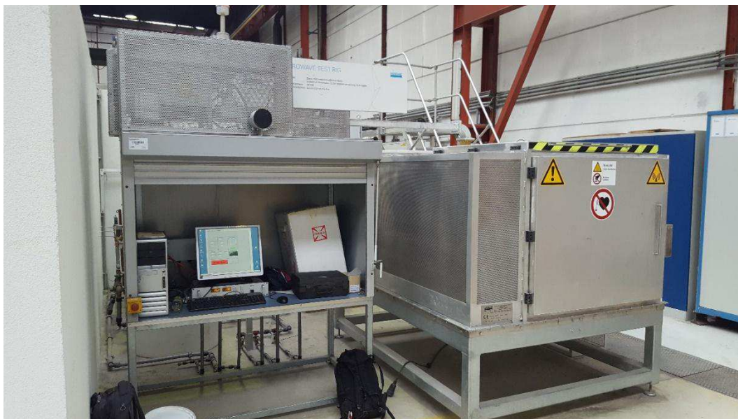
Figure 25: Microwave machine for large scale testing (Sandvik company).
