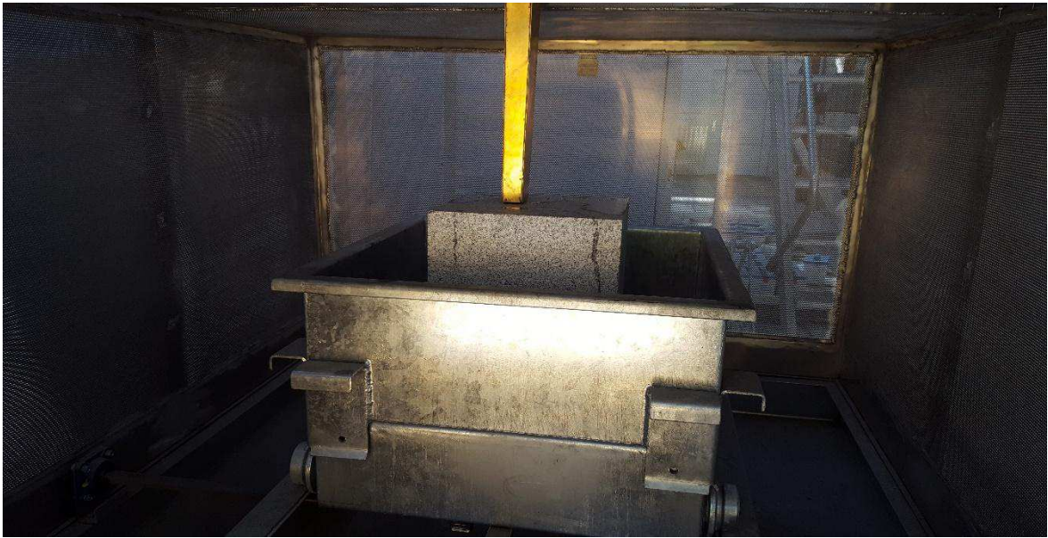
Figure 33: Placing the cube on platform and position of the waveguide on the sample.
