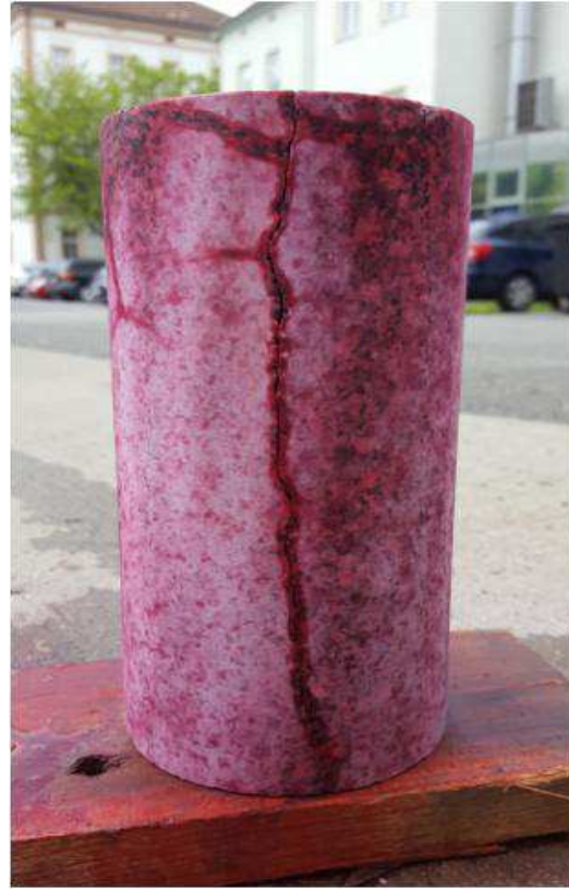
Figure 40: Preparing core for Computer Tomography.
