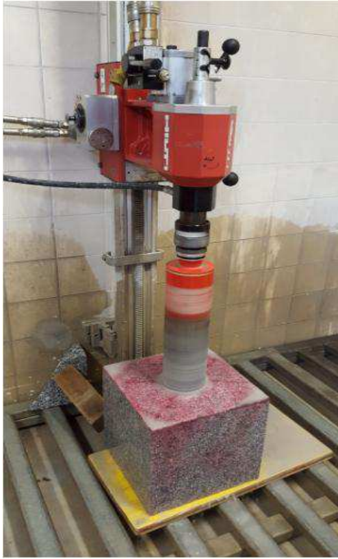
Figure 40: Preparing core for Computer Tomography.
