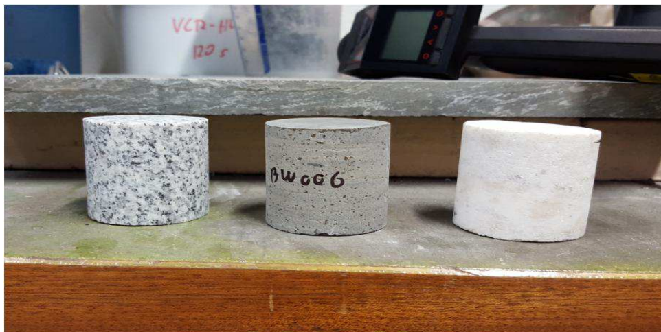
Figure 16: Samples for wave experiment (from left to right Granite, Volcanic rock, Marble).
