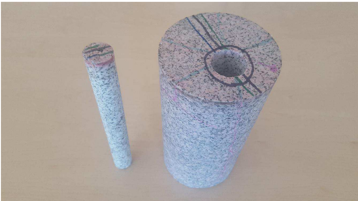
Figure 50: Drilled small core (2.5 cm diameter) with the center of the radiation spot.
