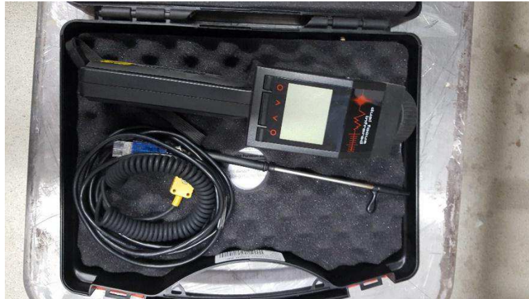
Figure 27: Infrared device for temperature measurement of samples.
