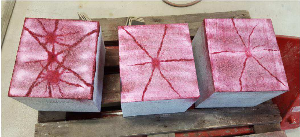
Figure 36: Surface of cube A, B and C after penetrating to highlight the cracks (from left to right).
