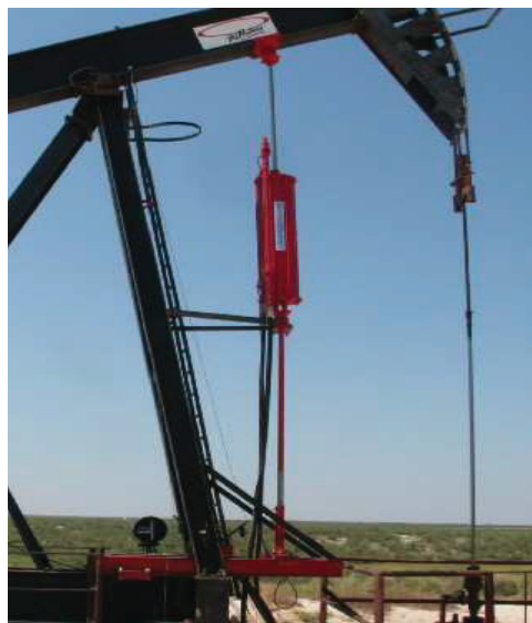
Figure 18: Conventional Unit with BMGC in front of the sampson post [22]
