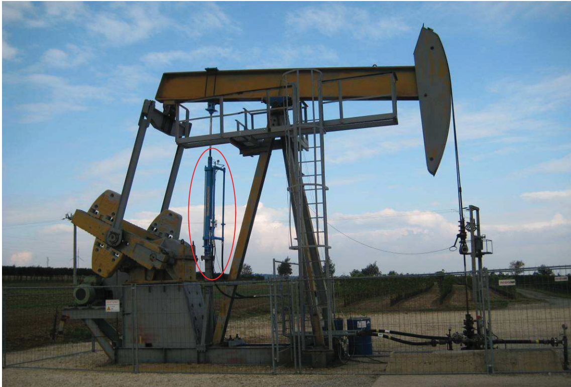
Figure 9: Beam Mounted Gas Compressor on a walking beam [20]
