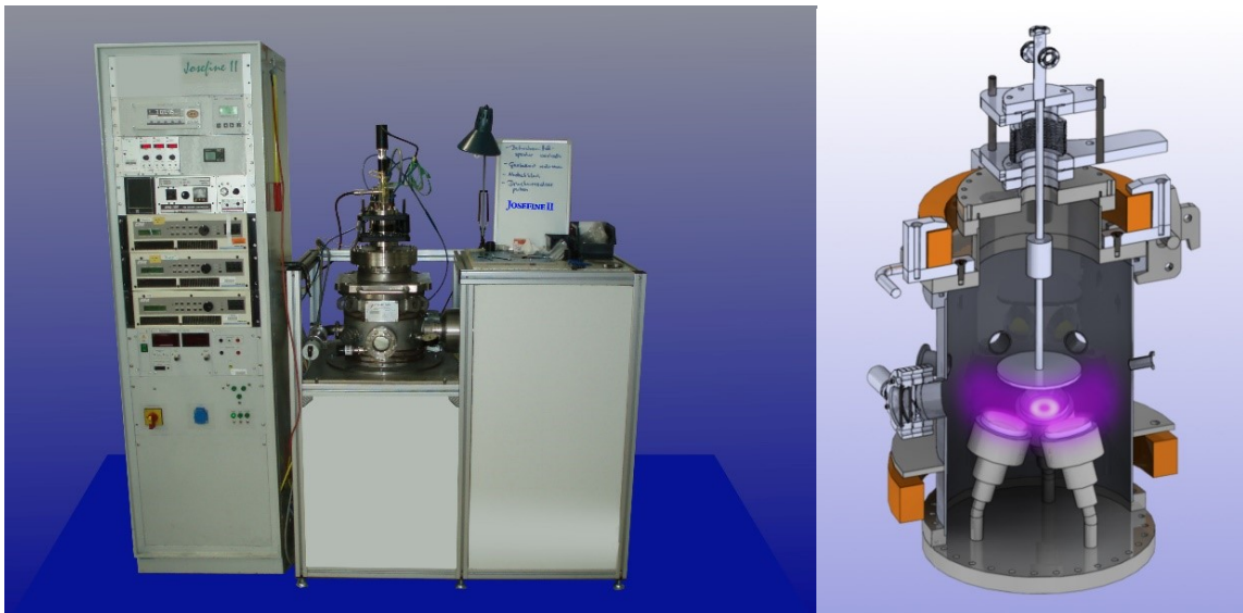
Figure 4.2: Laboratory-scale deposition plant with three targets used for film synthesis in Section 6 (own working group).
